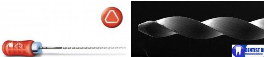
Figure 11 : Flexoreamer® (source : Dentsply-Maillefer) vue au MEB (<http://3.bp.blogspot.com/-HXRAYZDDaOc/T9TJQuJwDUI/AAAAAAAAACyU/byrsgyJ21pM/s1600/Picture6.jpg>)
