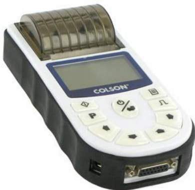
Electrocardiographe monopiste portable
