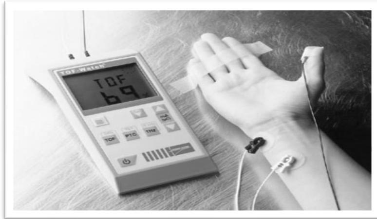
Figure 4: Accéléromyographe (TOF-Watch S®)
