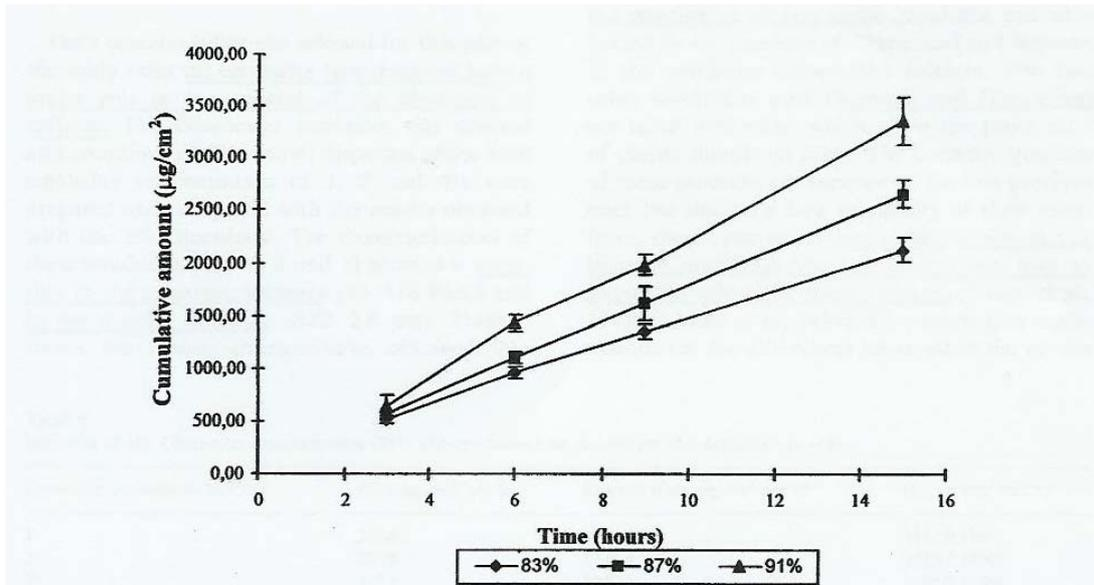
Fig. 6. Effect of the % dispersed phase (w/w) on the in vitro release profile of caffeine from concentrated emulsions obtained with 3% Glucoester emulsifier. (mean ± S.D.).
