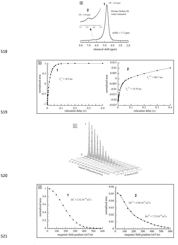
Figure 1. <sup>1</sup>H-NMR experiments in the water-saturated Nafion XL reinforced membrane (600 MHz).
