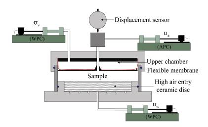
**Figure 1**. Suction controlled oedometer (APC: air pressure controller; WPC: water pressure controller).
