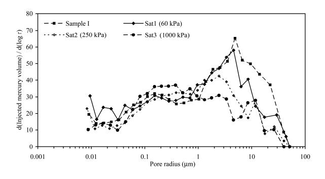
**Figure 9**. Samples fabric modification during a mechanical loading performed under saturated state (values in brackets indicate the maximum applied net stress).
