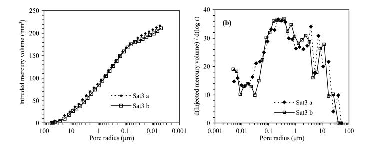
Figure 3. Test of MIP repeatability with sample Sat3: (a) mercury injection curves; (b) PSD.
