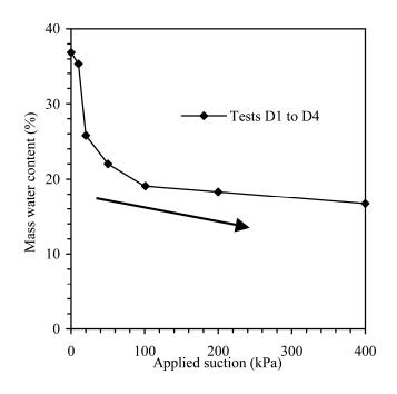
Figure 5. Soil-water characteristic curve of the tested samples.
