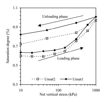
Figure 11. Variation of the saturation degree during loading in tests Unsat1 and Unsat2.
