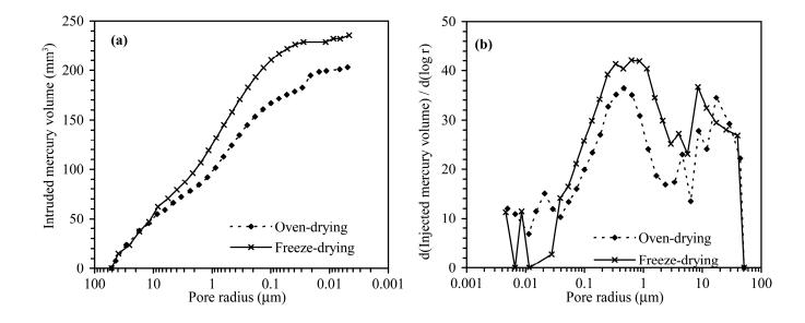
**Figure 4**. Drying procedure influence on MIP result for sample D2: (a) mercury injection curves; (b) PSD.
