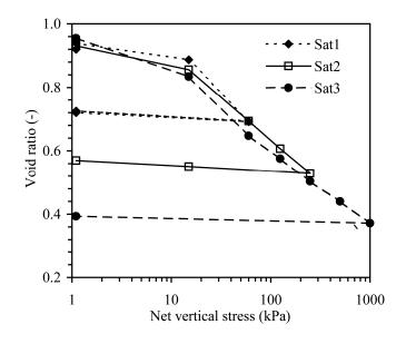
Figure 8. Results of the oedometer tests performed under saturated state (tests Sat1 to Sat3).
