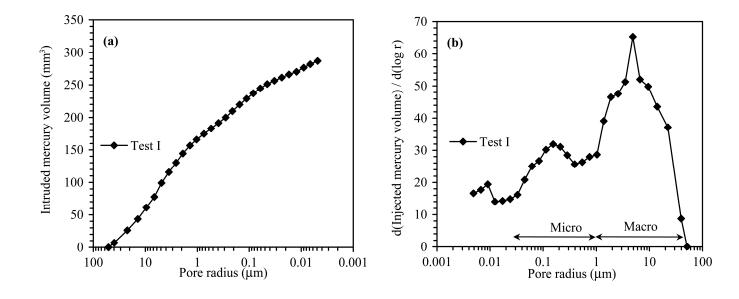
**Figure 6**. Fabric of sample I (initial state of the samples): (a) mercury injection curves; (b) PSD.
