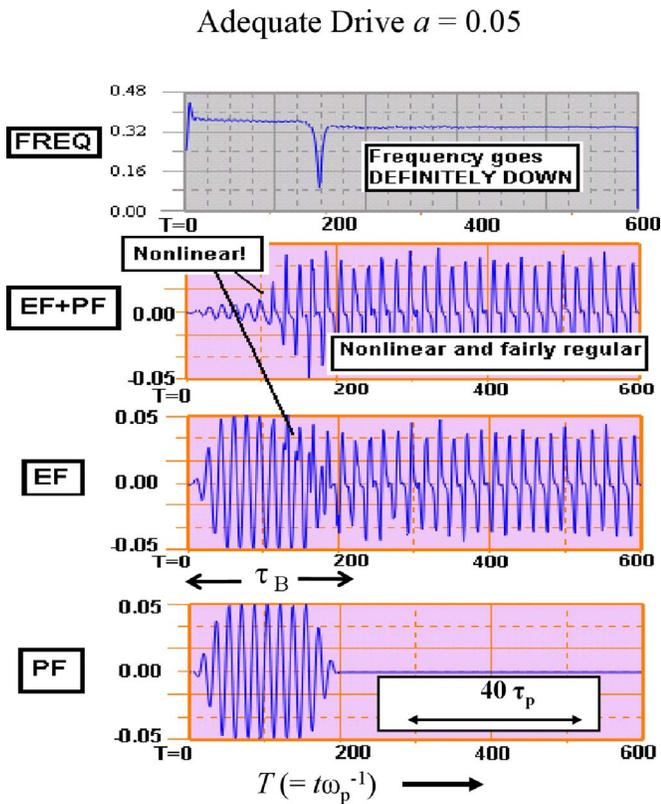
FIG. 2. (Color online) Successful KEEN results similar to Fig. 3 except the drive is now adequate ( $a=0.05$ ), with the trapping time  $\tau_B$  (shown by the double-headed arrow) being about equal to the drive duration. Now the result of the drive is to produce a long-lived KEEN wave. As often happens with KEEN wave drive, the final frequency is slightly reduced from the drive frequency.
