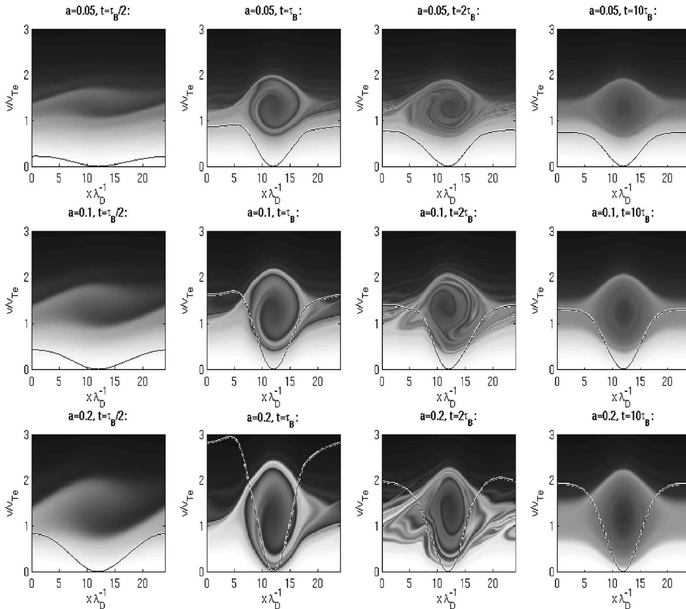
FIG. 7. Phase-space ( $X, V$ ) images of electron velocity distribution function during the drive-up period ( $t \leq \tau_B$ ) and after at the same times as for Fig. 6 (namely, at  $t/\tau_B = 1/2, 1, 2, 10$ ). The total-force potential profiles for each time frame are superposed for convenience.
