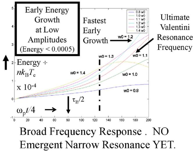
FIG. 12. (Color online) Time history of KEEN wave energy accumulation from the drive for different driving frequencies, ranging from  $0.8 \omega_{EAW}$  to  $1.4 \omega_{EAW}$ . Valentini resonance before its emergence (i.e., at early times) shows normal early added energy growth with weak drive ( $a=0.0026$ ).  $\tau_B/2$  is about 80 on this coarse time step scale of  $320\omega_p^{-1}$ . (The weak drive continues to  $3500\omega_p^{-1}$  or about  $5\tau_B$ .)
