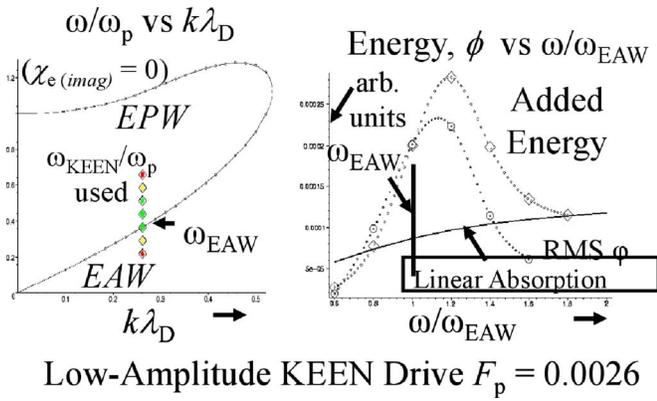
FIG. 10. (Color online) KEEN Amplitudes for  $k\lambda_D=0.26$ , with a common value for the low-amplitude drive ( $a=0.0026$ ) but with various drive frequency values. These correspond to  $\omega/\omega_p$  values from 0.2 to 0.7, corresponding to  $\omega/\omega_{EAW}$  values from 0.6 to 1.8. Note that, as expected from linear theory, KEEN waves can be produced over a broad range of frequencies for a given wavevector and do not show a narrow resonance around  $\omega_{EAW}$ .
