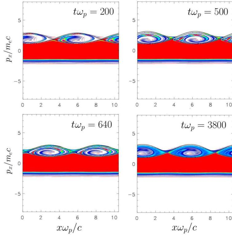
Figure 3: For a periodic SRS-F case, phase space representation of the electron distribution function corresponding to the situation shown in Fig. 2 when a small hot electron population is introduced initially. SRS-F enters now in a weak “kinetic” regime characterized by a small trapped electron population localized inside the wave-pulsating separatrices calculated using the data of the electrostatic potential given by the code.
