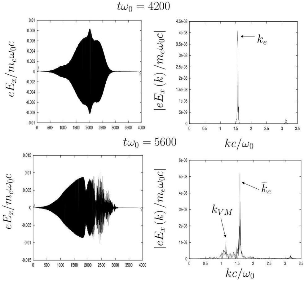
Figure 8: For SRS-B in optical mixing and for the parabolic plasma simulation of Fig. 7, we show here the longitudinal electric field vs  $x\omega_0/c$  at two different times, together with their  $k$ -spectra. Notice the increase in the wave number  $\tilde{k}_e$  at  $t\omega_0 = 5600$  (bottom right panel) from the initial  $k_e$  value to a larger value of  $\tilde{k}_e$ . This is due (see text) to a Langmuir Morales-O’Neil (LMO) shift with intensity.
