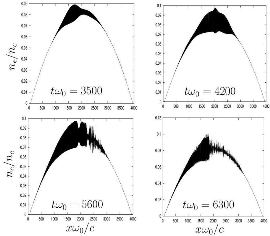
Figure 7: For the parabolic profile (maximum density of  $n_0 \simeq 0.0825n_c$ ,  $a_{osc} = 0.025$  and  $T_e = 2keV$ ) the typical density behavior at four different times. At  $t\omega_p = 3500$  the probe amplification breaks the symmetry of the interaction with respect to the top of the parabolic profile. At  $t\omega_p = 6300$  the lose of coherence of the shape for the electron density as the result of the pairwise vortex merging in that region.
