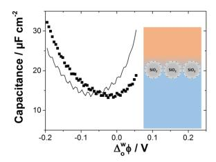
Figure 2: Potential dependence of the interfacial capacitance for the blank cell (solid line) and for ( $\blacksquare$ ) 0.5 g L<sup>-1</sup> of silica nanoparticles with a denser aqueous phase. Electrochemical cell 4.
