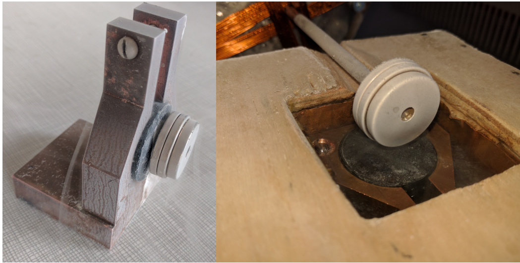
FIGURE 5.7: Paliers aimant-pastille supraconductrice
