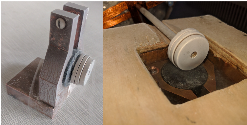
FIGURE 5.7: Paliers aimant-pastille supraconductrice
