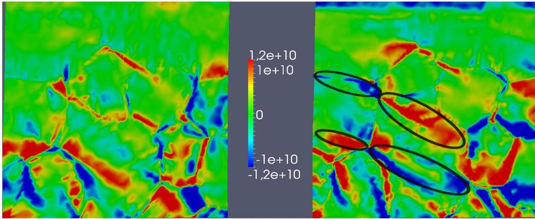
**Figure 14.** Distribution of screw (left) and edge (right) GND densities in  $m^{-2}$  on the first basal slip system at  $-1\%$  macroscopic strain. The black circles indicate the presence of opposite edge dislocation densities in grains 3 and 7 that bound the observed kink band.
