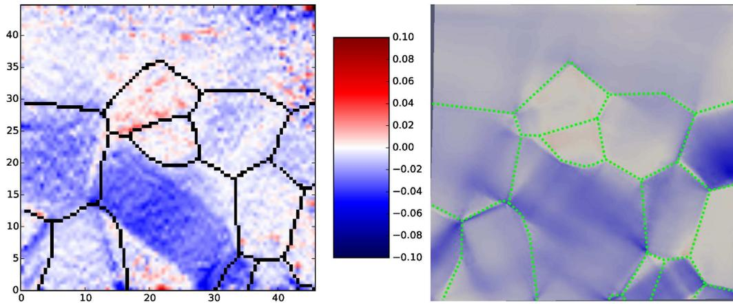
**Figure 7.** Distribution of strain  $\varepsilon_{yy}$  at  $-1\%$  of macroscopic strain: DIC measurement (left) and RPMFDM (right). The initial positions of the grain boundaries are indicated in black (left) or in dotted green lines (right). The dimensions of the sample are given in mm.
