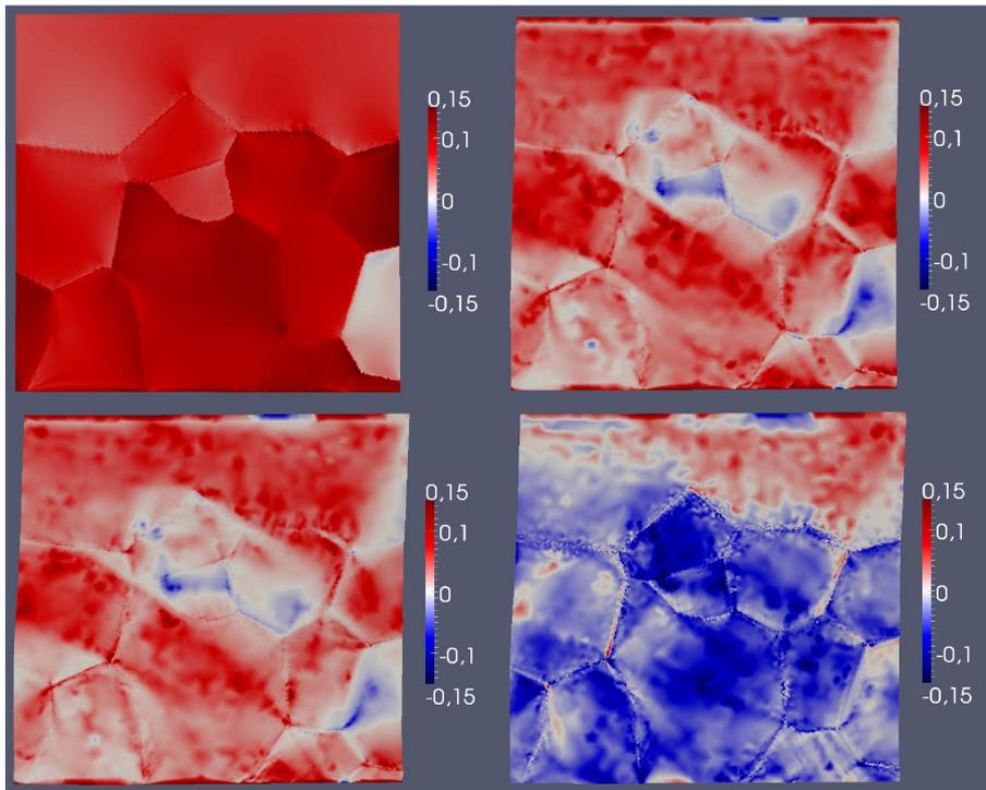
**Figure 16.** Distribution of the resolved shear stress in *MPa* on the basal slip system numbered 1,  $\tau^{(1)}$ , just after loading, at  $-1\%$  of macroscopic strain, just before unloading at  $-1.9\%$  of macroscopic strain and just after unloading (from left to right and top to bottom, respectively).
