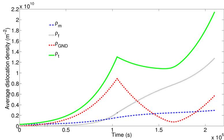
**Figure 5.** Evolution of the statistical mobile ( $\rho_m$ ), immobile ( $\rho_f$ ), GND ( $\rho_{GND}$ ) and total ( $\rho_t$ ) dislocation densities, summed over all slip systems and averaged over the specimen, during torsion creep of single crystal A.
