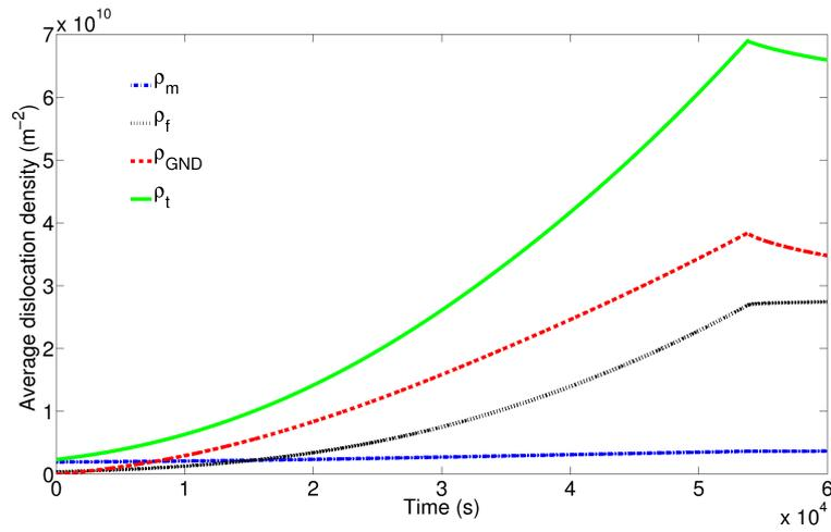
**Figure 11.** Evolution of the statistical mobile ( $\rho_m$ ), immobile ( $\rho_f$ ), GND ( $\rho_{GND}$ ) and total ( $\rho_t$ ) dislocation densities, summed over all slip systems and averaged over the specimen, during compression creep of the multi-crystal.
