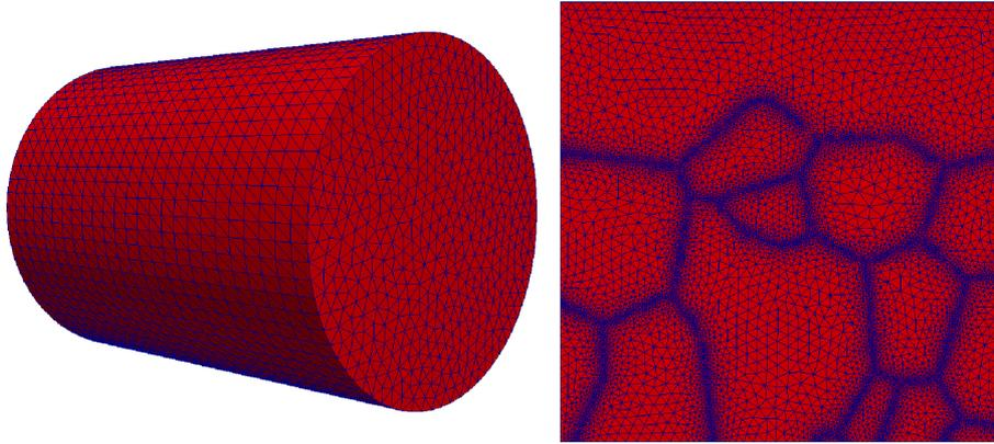
**Figure 2.** Unstructured FE mesh used in the simulations: single crystal A (left) with dimensions 46 mm (diameter) \* 50 mm (height) and multi-crystal (right) with dimensions 47.7 mm (height) \* 48 mm (width) \* 1.2 mm (thickness).
