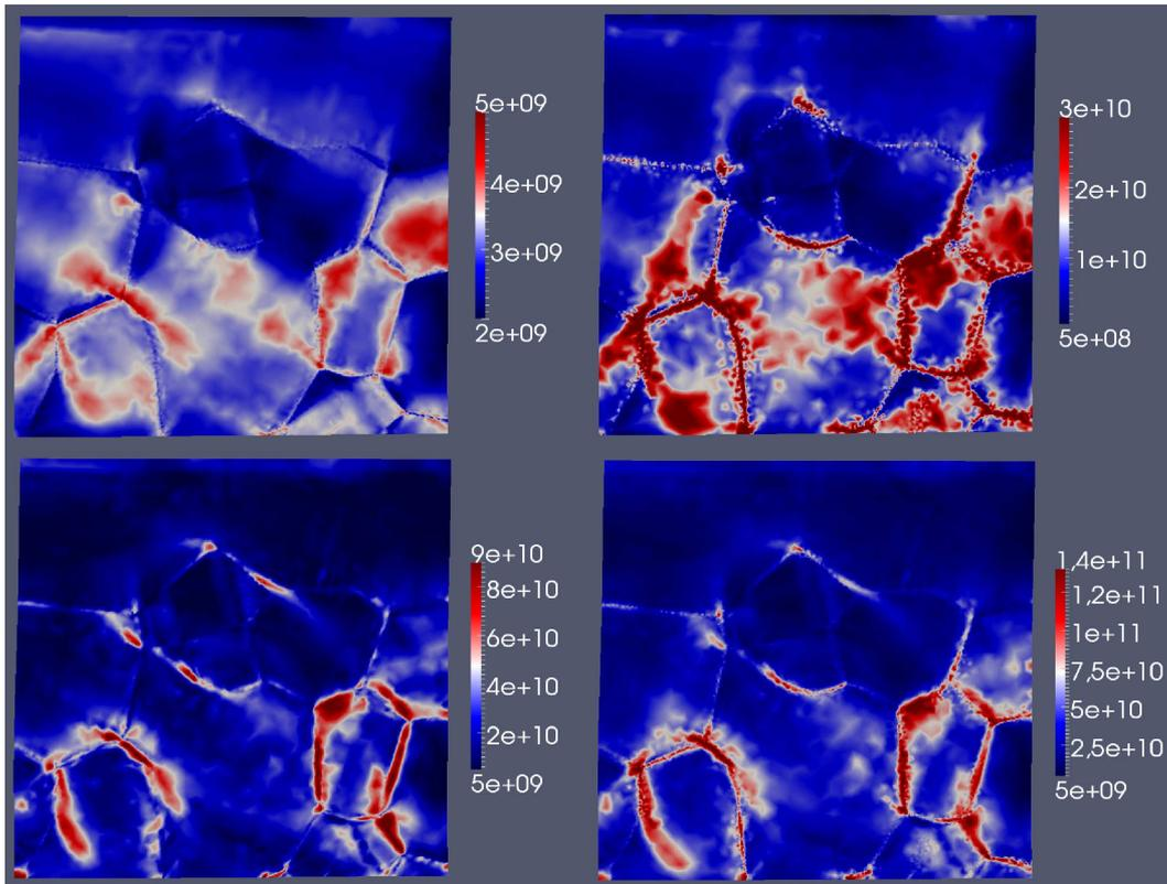
**Figure 12.** Distribution of the mobile SSD ( $\rho_m$ ), immobile SSD ( $\rho_f$ ), GND ( $\rho_{GND}$ ) and total ( $\rho_t$ ) dislocation densities in  $m^{-2}$ , summed over all slip systems, at  $-1\%$  macroscopic strain (from left to right and top to bottom, respectively).
