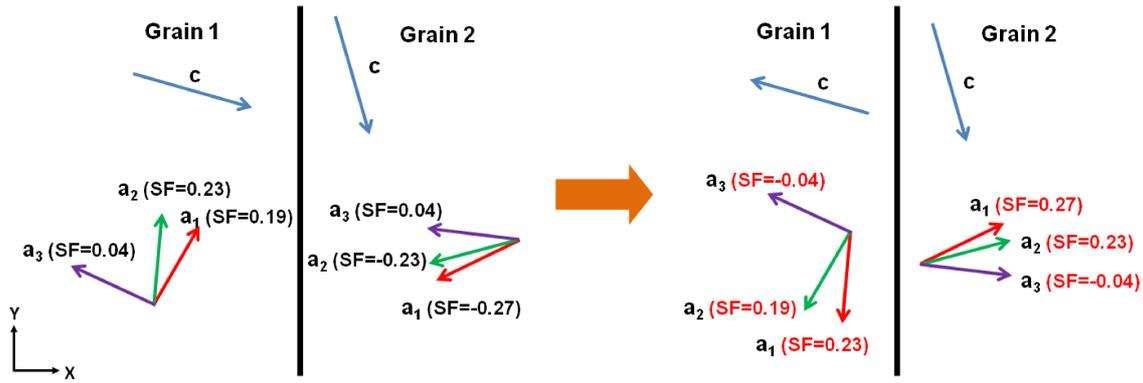
**Figure 1.** Scheme illustrating the re-numbering of basal slip systems in order to resolve the transport equations on slip systems at grain boundaries. The arrows represent the projections of the  $c$ -axis and the 3  $a$ -axis of the hexagonal lattice in the global plane  $(x, y)$ . SF denotes Schmid Factor. The values correspond to grain 1 and 2 of the compressed ice multi-crystal (see figure 3).
