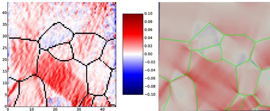
**Figure 8.** Distribution of strain  $\varepsilon_{xx}$  at  $-1\%$  of macroscopic strain: DIC measurement (left) and RPMFDM (right). The initial positions of the grain boundaries are indicated in black (left) or in dotted green lines (right). The dimensions of the sample are given in mm.
