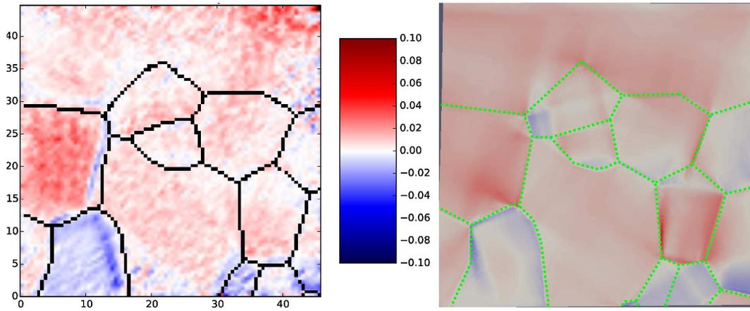
**Figure 9.** Distribution of strain  $\varepsilon_{xy}$  at  $-1\%$  of macroscopic strain: DIC measurement (left) and RPFDM (right). The initial positions of the grain boundaries are indicated in black (left) or in dotted green lines (right). The dimensions of the sample are given in mm.
