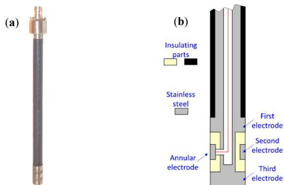
Figure 1. Submersible dielectric probe (SDP): (a) Photograph, (b) Schematic representation.
