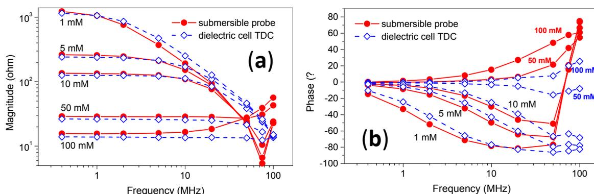
**Figure 3.** Comparison of the dielectric response of the submersible probe with that of a classic thermostatable dielectric cell for increasing concentrations of NaCl in the 1 to 100 mM range: (a) Magnitude; (b) Phase.
