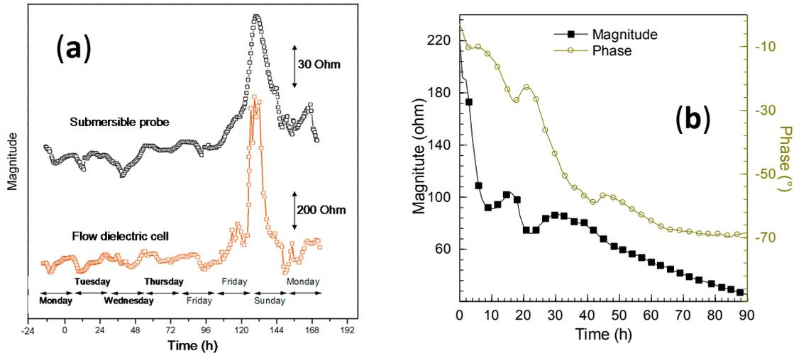
**Figure 4.** Real-time monitoring of the activated sludge in a pilot reactor (measurements made at 0.4 MHz): (a) usual changes of the dielectric parameters for a week by means of the submersible probe (SDP) and a flow dielectric cell (FDC); (b) after the road salting in wintertime with the SDP.
