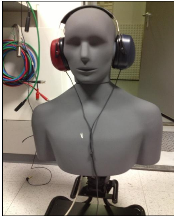
Figure 25: Knowles Electronic Manikin for Acoustic Research (KEMAR)
