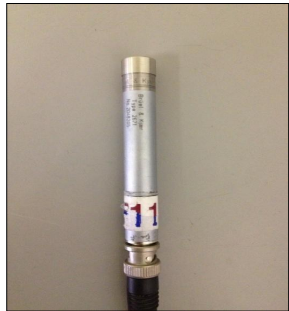
Figure 45: Microphone B&K de type 4189 noté F11
