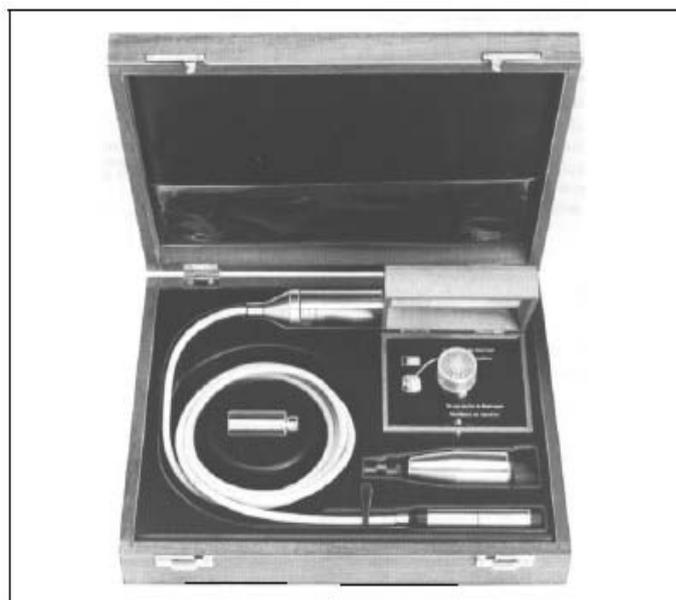
Brüel & Kjær has developed the 1" Condenser Microphone Type 4179 and Microphone Preamplifier Type 2660 system for measuring ultra-low sound pressure levels. High-quality, conventional 1" condenser microphones, such as B&K Types 4144 and 4145, and half-inch diameter Types 4165 and 4166, provide for the majority of noise measurements to IEC, ISO
