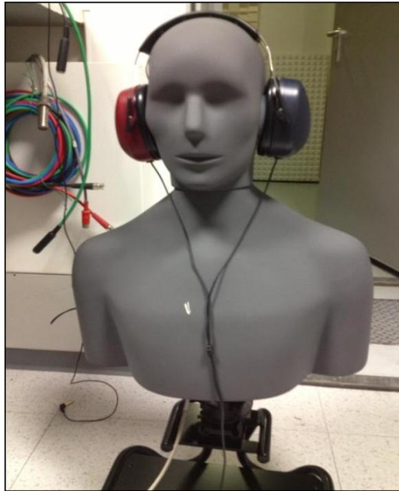
Figure 25: Knowles Electronic Manikin for Acoustic Research (KEMAR)
