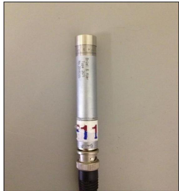
Figure 45: Microphone B&K de type 4189 noté F11
