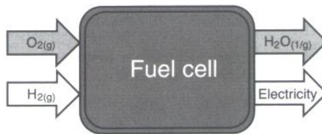
Fig. I.1 - General concept of a hydrogen–oxygen (H 2 –O 2 ) fuel cell. [1]
