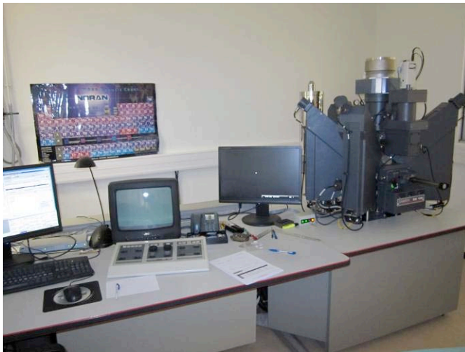
Figure 11 : Microsonde de Castaing CAMECA® SX 100
