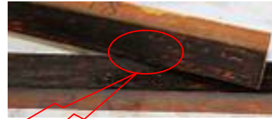
Figure 20 the broken welding joint with No.2 tannin solution after in the cold water
