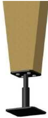
Figure 13: Assemblage poteau bois-pied de poteau
