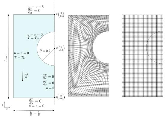
**Figure 5**: Sketch of the computational domain for the natural convection test-case (with  $L=1\,\mathrm{m}$ ,  $T_{\mathrm{H}}=1\,\mathrm{K}$ ,  $T_{\mathrm{C}}=0\,\mathrm{K}$ ), curvilinear mesh L1 and Cartesian mesh M1 of size  $32\times64$  used respectively for the FLUENT<sup>©</sup> and LS-STAG computations.
