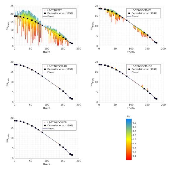
**Figure 7**: Profiles of the Nusselt number along the half cylinder for the various discretization of diffusion in the LS-STAG method, and comparison with the FLUENT<sup>©</sup> computation and reference results of Demirdžić *et al* [9]. The profiles are colorized with respect to the volume-change ratio  $RV_{i,j}$  (18) of the cut-cells.
