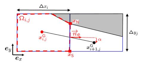
Figure 2: Relevant notations used for the discretization of the diffusion flux at the east face of cut-cell  $\Omega_{i,j}$ .
