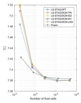
Figure 6: Convergence of the average Nusselt number with respect to the number of fluid cells.
