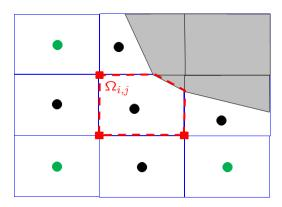
Figure 3: Stencil used for the discretization of diffusion in cut-cell  $\Omega_{i,j}$ . In black: 5-point stencil for 2-point discretization. For the DCM discretization with reconstruction at vertices ( $\blacksquare$ ), unknowns at the green centroids are added to the stencil.
