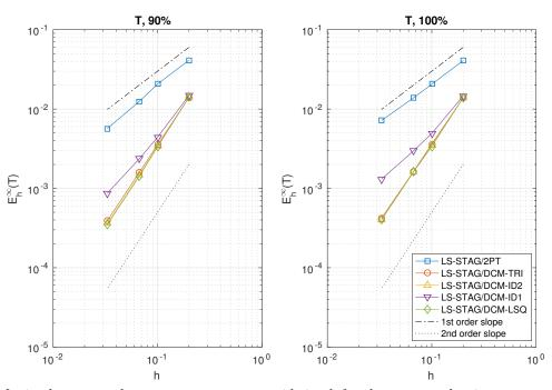
**Figure 4**: Maximal error on the temperature versus grid size h for the pure conduction test case. At left : on 90% of the domain, at right : on the whole domain.
