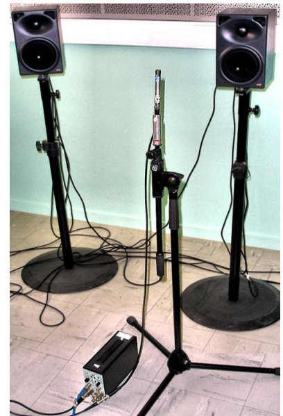
Figure 3.1 Installation du microphone demi-pouce
