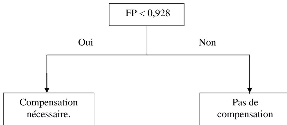
**Figure 2:** Condition de compensation.
