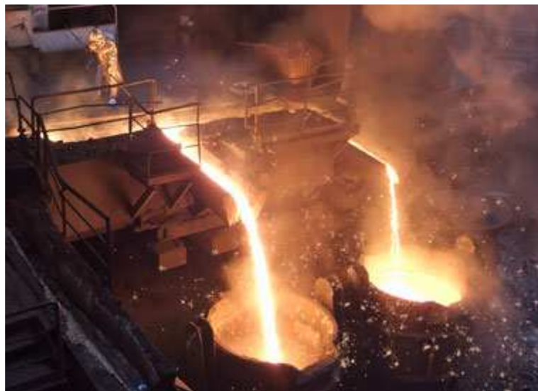
Figure 1.3 : Haut-fourneau - Coulée de fonte
