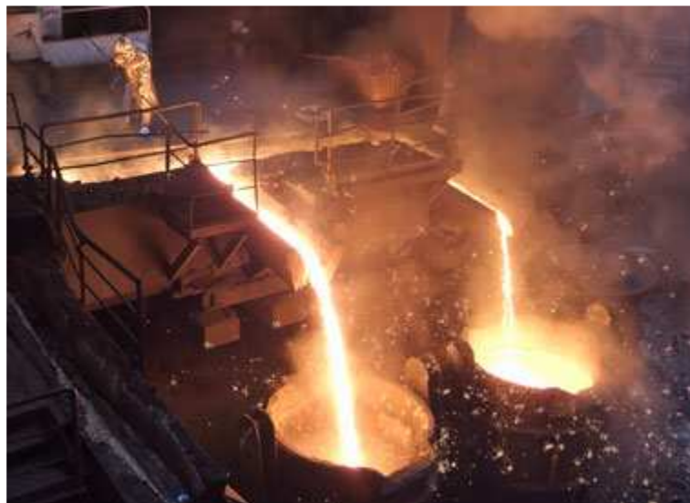
Figure 1.3 : Haut-fourneau - Coulée de fonte
