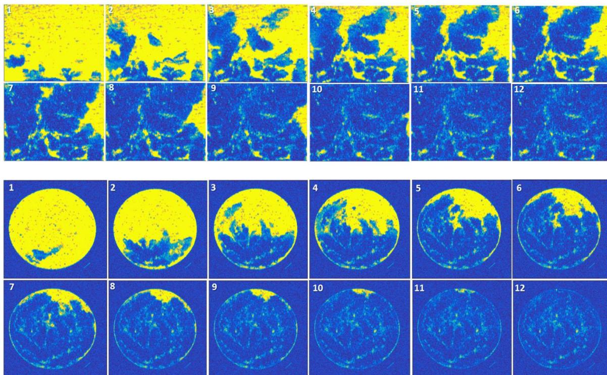
**Figure 5:** Consecutive MRI images of the water–oil displacement in the model of packed sand column with the injection flow rate of 0.06 ml/min. The time interval between each image equals 15 minutes.
