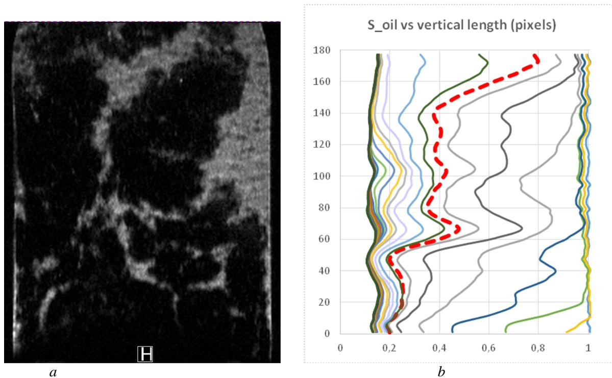
**Figure 6:** Oil saturation distribution in the packed sand model, the injection flow rate is 0.06 ml/min: (a) MRI image of displacement process after 2h of injection, (b) variation of oil saturation vs vertical coordinate in time, red dashed line corresponds to the saturation profile for the image (a).
