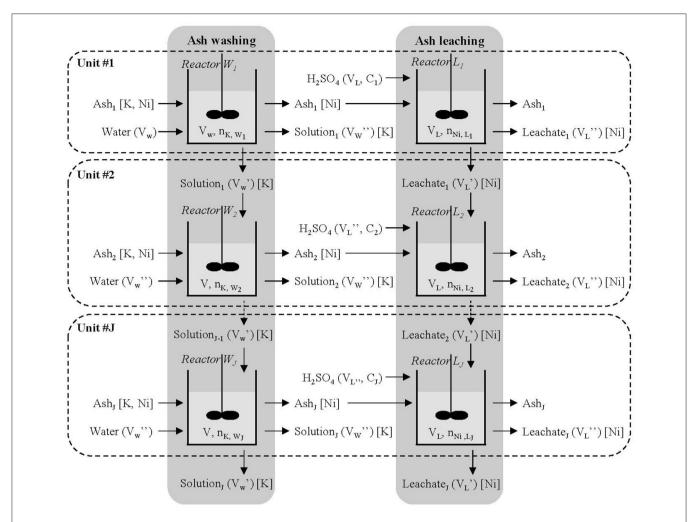
FIGURE 7 | Parallel batch configuration for Odontarrhena muralis s.l. ash washing and leaching. Liquid properties are indicated in brackets and targeted elements in square brackets.
