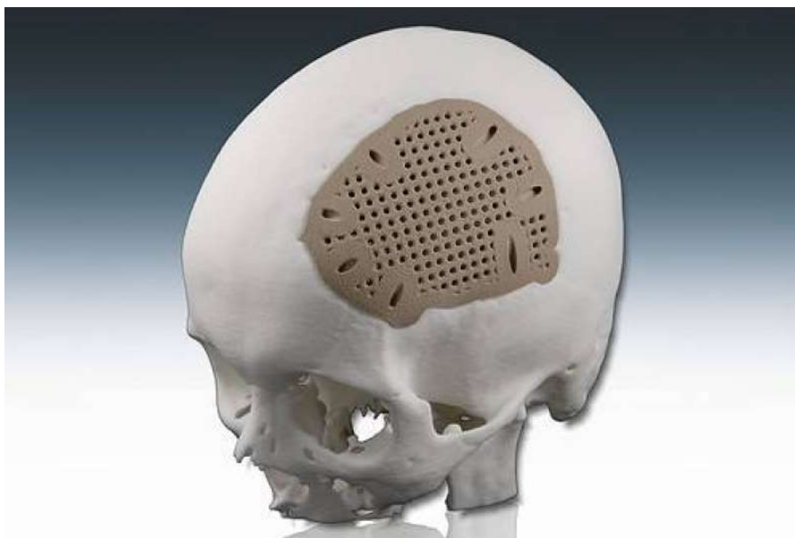
Figure 150 : Volet crânien imprimé en PEEK HP3 (Source : Foletti & Al. 2012)
