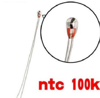
Figure 89 : Thermistance NTC 3950 - 100k (Source : a2itronic)
