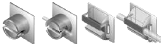
Figure 3: (A) Attache de Ford, (B) Attache de Boyd, source : (Ludwig and Bister 2011)
