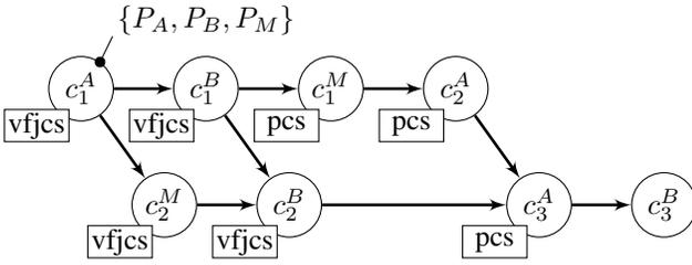
Figure 7. Mallory ( $P_M$ ) is provably malicious. She is known as evicted in  $c_3^A$ . Since  $c_3^A$  is provably causally stable (pcs), then Mallory is no longer a required observer of any contributions.  $c_2^B$  precedes  $c_2^A$  and are pcs. Thus Alice ( $P_A$ ) and Bob ( $P_B$ ) are provably linear observers of  $c_2^B$  and all preceding contributions. These contributions have only Alice and Bob as required observers. They are thus view-fork-join-causally stable (vfjcs).
