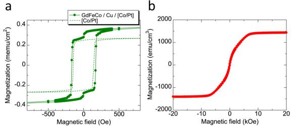
Figure S1: a, Magnetic curves for GdFeCo / Cu / [Co/Pt] sample and [Co/Pt] sample measured by SQUID-VSM. b, In-plane magnetization curve for [Co/Pt] film. Slope correction was performed to subtract diamagnetic contribution of the substrate and sample holder.
