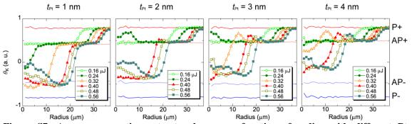
Figure S7: Average magnetic contrast values as a function of radius with different Pt layer thicknesses. Solid lines are the average values of the initial states and symbols are the values after 1<sup>st</sup> fs-laser pulse is irradiated.
