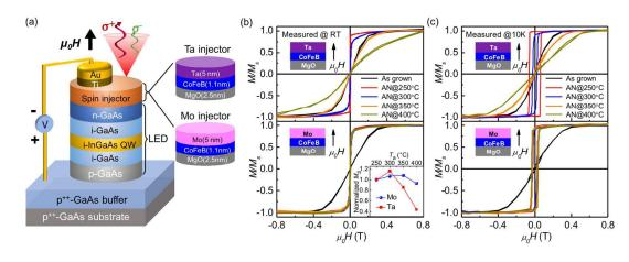
**Figure 1.** Magnetic characterization of spin-injectors. (a) Schematics of spin-LED structure with Ta or Mo capped spin-injector. (b) M-H curves measured at RT for Ta and Mo spin-injectors before and after annealed at different temperatures. For short, "AN" represents for annealing. Inset: normalized  $M_s$  of Ta and Mo spin-injectors at RT as a function of annealing temperature. (c) M-H curves measured at 10K for Ta and Mo spin antealed at different temperatures.
