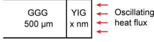
FIG. 1. The sketch of the samples GGG (500 \mu\text{m} )/YIG ( x nm) where x = 50, 270, and 2800 . An oscillating heat flux is applied on the surface.
