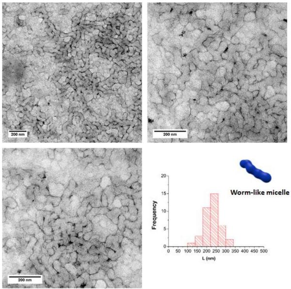
**Figure S17.** TEM images of Dex- $g^5$ -PHPMA<sub>340</sub> nanostructures prepared by photo-PISA of HPMA in aqueous medium using Dex-TTC as the macro-CTA, at 5% w/w solids content.
