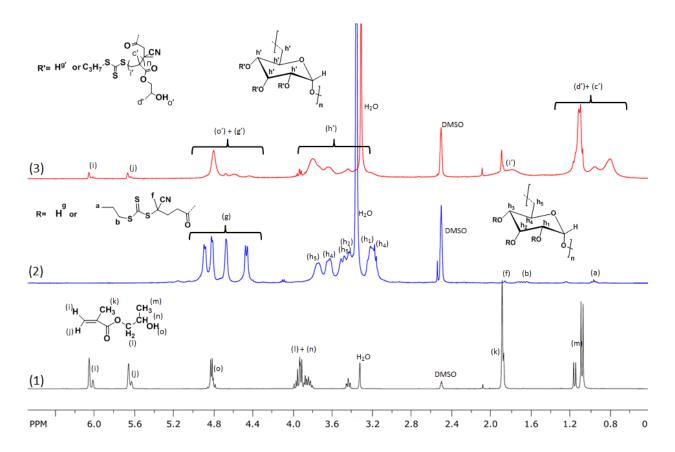
**Figure S7.** <sup>1</sup>H NMR spectra of (1) HPMA monomer, (2) Dex-TTC and crude Dex-g<sup>5</sup>-PHPMA<sub>340</sub> glycopolymer prepared by photo-PISA of HPMA in aqueous medium using Dex-TTC as the macro-CTA, at 5% w/w solids content.
