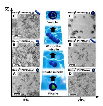
**Fig. 3.** TEM images of a series of Dex- $g^5$ -PHPMA<sub>Y</sub> based glyconanostructures prepared by aqueous photo-PISA of HPMA using Dex-TTC as the macro-CTA, at room temperature and with two solids contents (5% and 20% w/w) and y as targets. Samples were observed at 1 mg.mL $^{-1}$ .
