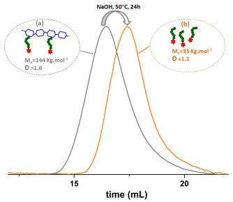
**Figure S10.** SEC traces of glycopolymers Dex-g<sup>5</sup>-PHPMA<sub>180</sub> (a) and corresponding cleaved PHPMA grafts obtained by treatment in alkaline conditions at 50°C during 24 hours.
