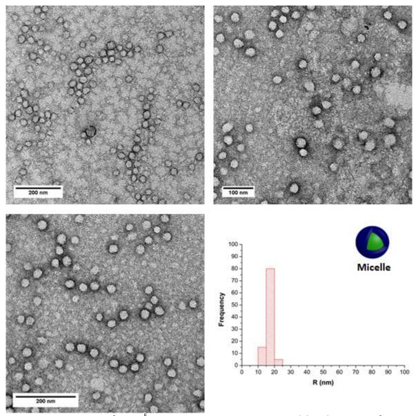
**Figure S18.** TEM images of Dex- $g^5$ -PHPMA<sub>105</sub> nanostructures prepared by photo-PISA of HPMA in aqueous medium using Dex-TTC as the macro-CTA, at 20% w/w solids content. The histogram was made from TEM images based on 100 nano-objects.
