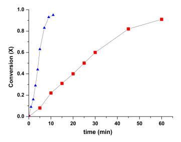
**Figure S8.** Evolution of conversion with time of aqueous HPMA photo-PISA performed at (■) 5% w/w and (▲)20% w/w solids content using Dex-TTC as the macro-CTA.[HPMA]<sub>0</sub>/[TTC]<sub>0</sub>=190/1.
