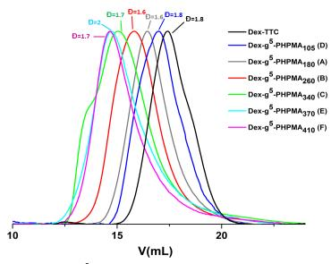
**Figure S9.** SEC traces of various Dex- $g^5$ -PHPMA<sub>y</sub> prepared by aqueous photo-PISA of HPMA using Dex-TTC as the macro-CTA, at a solids concentration of 5% w/w solids content for (A, B and C), and at 20% w/w solids content for (D, E and F).
