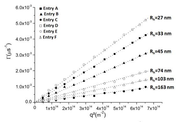
**Figure S14.**  $q^2$  dependence of the relaxation rate ( $\Gamma$ ) for various Dex- $g^5$ -PHPMA, nanostructures prepared by photo-PISA of HPMA in aqueous medium using Dex-TTC as the macro-CTA, at different conditions (see Table S1).
