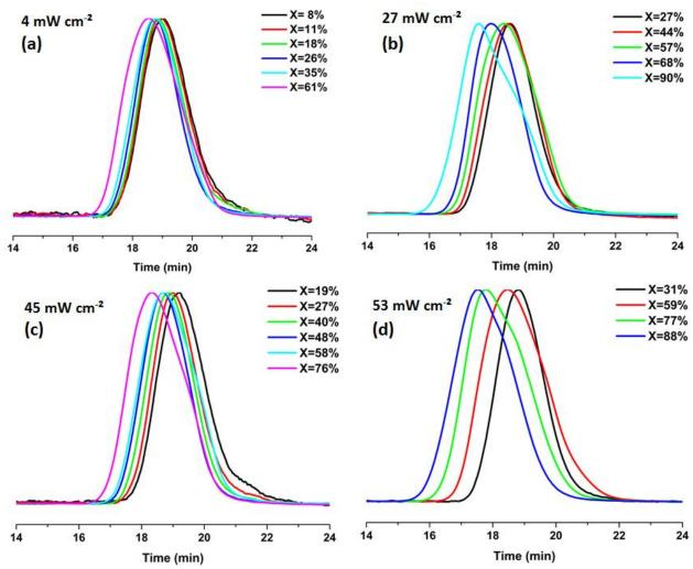
**Figure S3.** Evolution of PHPMA SEC traces (LS detection, DMF/LiCl at 50°C) with conversion (X). PHPMA were prepared by RAFT polymerization of HPMA at room temperature in DMSO using TTC (1) with various UV lamp intensities: (a) 4 mW/cm<sup>-2</sup>, (b) 27 mW/cm<sup>-2</sup>, (c) 45 mW/cm<sup>-2</sup> and (d) 53 mW/cm<sup>-2</sup>. [HPMA]<sub>0</sub>/[TTC]<sub>0</sub>=300/1.
