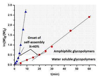
Fig. 1. Kinetics of the aqueous HPMA photo-PISA performed at (■) 5% w/w and (▲)20% w/w solids content using Dex-TTC as the macro-CTA.[HPMA]₀/[TTC]₀=190/1.
