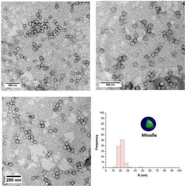
**Figure S15.** TEM images of Dex-g<sup>5</sup>-PHPMA<sub>180</sub> nanostructures prepared by photo-PISA of HPMA in aqueous medium using Dex-TTC as the macro-CTA, at 5% w/w solids content. The histogram was made from TEM images based on 100 nano-objects.
