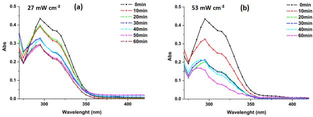
**Figure S4.** Evolution of UV-Vis absorbance spectra of TTC (1) in DMSO ([TTC]= 0.1 mM) under various UV irradiation intensities. (a)27mW.cm<sup>-2</sup> and (b) 53mW.cm<sup>-2</sup>) at different times.
