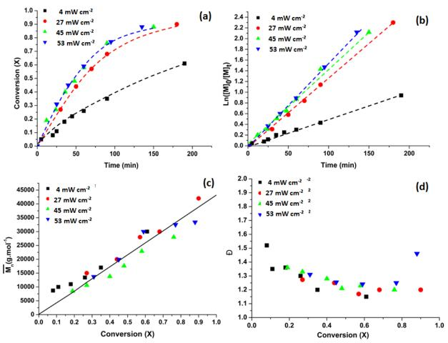
**Figure S2.** RAFT homopolymerization of HPMA in DMSO at room temperature, using TTC (1) with various UV lamp intensities (4 mW/cm<sup>-2</sup>, 27 mW/cm<sup>-2</sup>, 45 mW/cm<sup>-2</sup> or 53 mW/cm<sup>-2</sup>). [HPMA]<sub>0</sub>/[TTC]<sub>0</sub>=300/1. Plots of (a) conversion and (b)  $\ln[M]_0/[M]_t$  versus time. Plots of (c)  $\overline{M}_n$  and (d)  $\Phi$  versus conversion.
