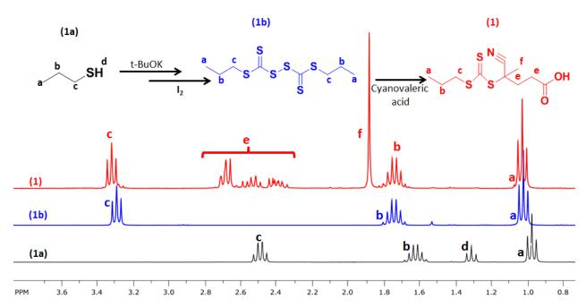
**Figure S1.** <sup>1</sup>H NMR spectra of 1-propanethiol (1a), bis-(propanesulfyanyl thiocarbonyl) disulfide (1b) and 4-(propylthiocarbonothioylthio)-4-cyanopentanoic acid (TTC) (1) in CDCl<sub>3</sub>.
