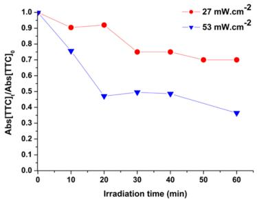
**Figure S5.** Degradation of TTC (1) in DMSO ([TTC]= 0.1 mM) under various UV irradiation intensities (27mW.cm<sup>-2</sup> and 53mW.cm<sup>-2</sup>), using the absorbance peak at 295nm (see figure S4).
