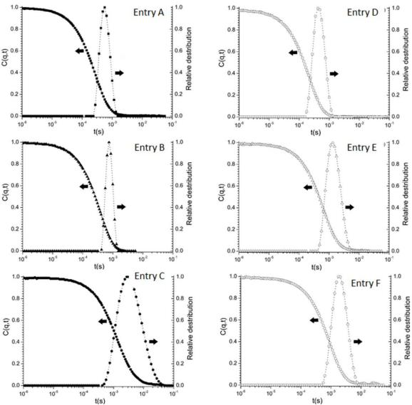
**Figure S13.** Autocorrelation functions and size distributions recorded at scattering wave vectors q of  $1.7 \times 10^7 \text{ m}^{-1}$  for different Dex-g<sup>5</sup>-PHPMA<sub>y</sub> nanostructures prepared by photo-PISA of HPMA in aqueous medium using Dex-TTC as the macro-CTA, at different conditions (see Table S1).
