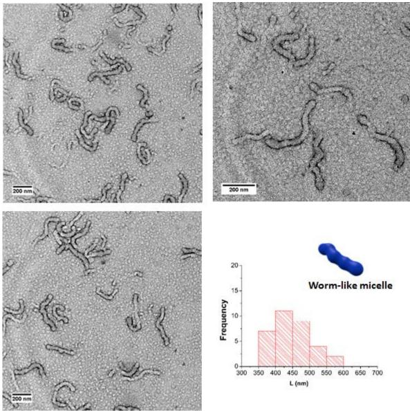
**Figure S19.** TEM images of Dex-g<sup>5</sup>-PHPMA<sub>370</sub> nanostructures prepared by photo-PISA of HPMA in aqueous medium using Dex-TTC as the macro-CTA, at 20% w/w solids content. The histogram was made from TEM images based on length (L) of 40 nano-objects.
