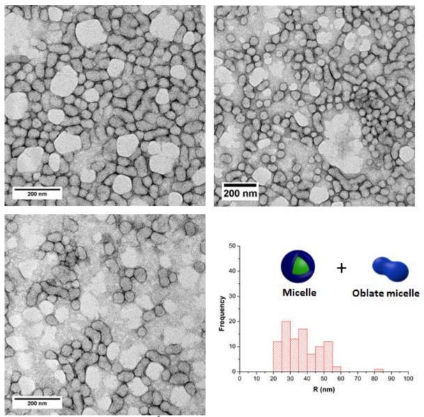
**Figure S16.** TEM images of Dex-g<sup>5</sup>-PHPMA<sub>260</sub> nanostructures prepared by photo-PISA of HPMA in aqueous medium using Dex-TTC as the macro-CTA, at 5% w/w solids content. The histogram was made from TEM images based on 100 nano-objects.
