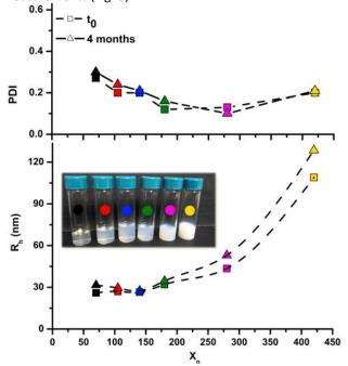
**Fig. 2.** Evolution of hydrodynamic radius (R<sub>h</sub>), PDI and visual inspection of the samples as a function of the grafts length  $(\overline{X_n})$ . Dex-g<sup>5</sup>-PHPMA $_Y$  colloidal dispersions were prepared at 5% w/w solids content, by photo-PISA of HPMA using Dex-TTC as the macro-CTA.
