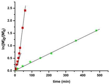
Figure S12. Kinetics of the aqueous HPMA photo-initiated RAFT performed in (■) water and ( ) DMSO at 5% w/w selids content using Dex-TTC as the macro-CTA.[HPMA]<sub>0</sub>/[TTC]<sub>0</sub>=190/1.
