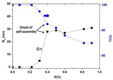
**Figure S11.** Evolution of (■) hydrodynamic radii (R<sub>h</sub>) and (•) transmittance (%) of gluco-nanostructure suspensions prepared via aqueous photo-PISA of HPMA using Dex-TTC as the macro-CTA, at a solids concentration of 5% w/w solids content. [HPMA]<sub>0</sub>/[TTC]<sub>0</sub>=190/1.
