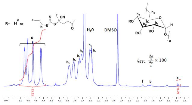
**Figure S6.** <sup>1</sup>H NMR spectrum of Dex-TTC (2).  $\zeta_{\text{TTC}}$  is the number of TTC moieties per 100 glucopyranosic units (here,  $\zeta_{\text{TTC}}$ =2.5).
