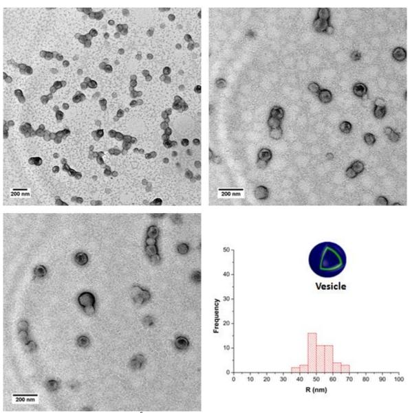
**Figure S20.** TEM images of Dex- $g^5$ -PHPMA<sub>410</sub> nanostructures prepared by photo-PISA of HPMA in aqueous medium using Dex-TTC as the macro-CTA, at 20% w/w solids content. The histogram was made from TEM images based on 50 nano-objects.
