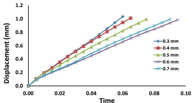
Fig. 7 Penetration depths related to each nozzle diameter
