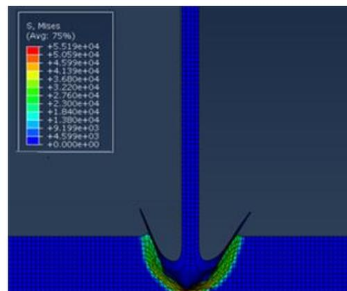
Fig. 3 A two-dimensional FEA model of the liquid jet penetrating into the soft target
