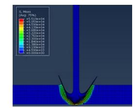
Fig. 3 A two-dimensional FEA model of the liquid jet penetrating into the soft target
