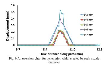
To make a clear measurement, a new plot has been generated (Fig. 10) that shows the X-axis from 8 mm to 12 mm long, which can be extracted that the maximum width of 2.5 mm was created by 0.7 mm nozzle followed by 0.6 mm nozzle that penetrated 2.2 mm of width. Meanwhile, the three smallest nozzle diameters had almost the same cutting width of 1.9 mm; therefore, 0.5 mm nozzle can be consider a better choice since it is easier to create and has the same effect on penetration width.
