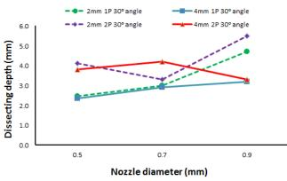
Fig. 6 Dissecting depth values for 30° angle parameter in experiment 2
