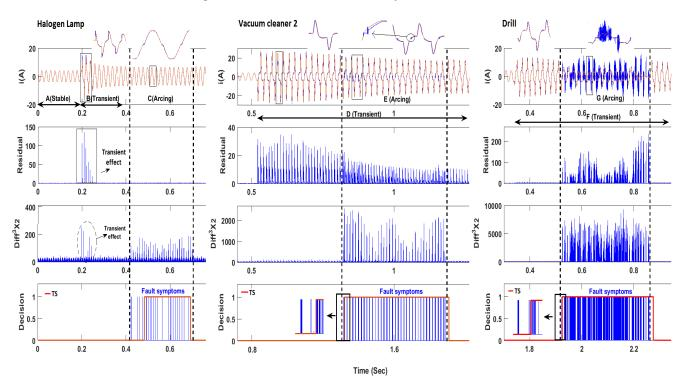
Figure 13: Sub-case 2: transient current (masking-type 1) of an halogen lamp, vacuum cleaner 2 and a drill.
