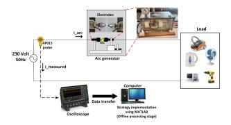
Figure 3: Experimental platform for series arc fault generation.
