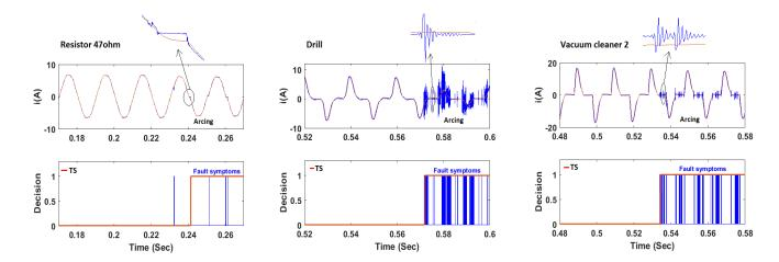
Figure 16: Sub-case 5: fault detection using an EMI filter.
