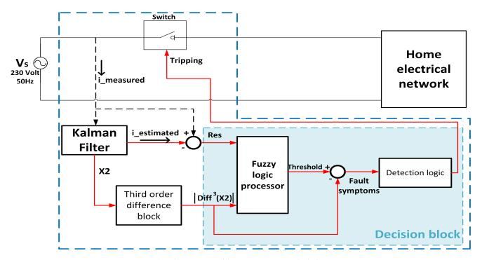
Figure 1: Scheme proposed for AC series arcing fault detection.
