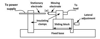
Figure 2: Arc generator by contact breakage.
