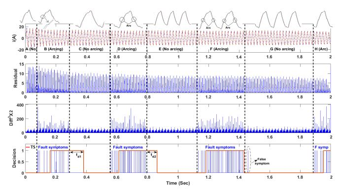
Figure 14: Sub-case 3: transient current (masking-type 2) of a drill.
