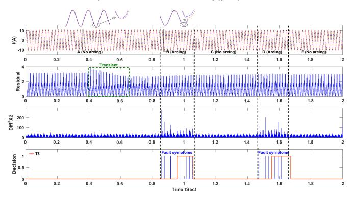
Figure 15: Sub-case 4: transient current (masking-type 3) of vacuum cleaner 2.
