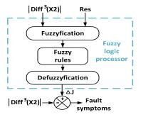
Figure 9: Fuzzy thresholding logic.
