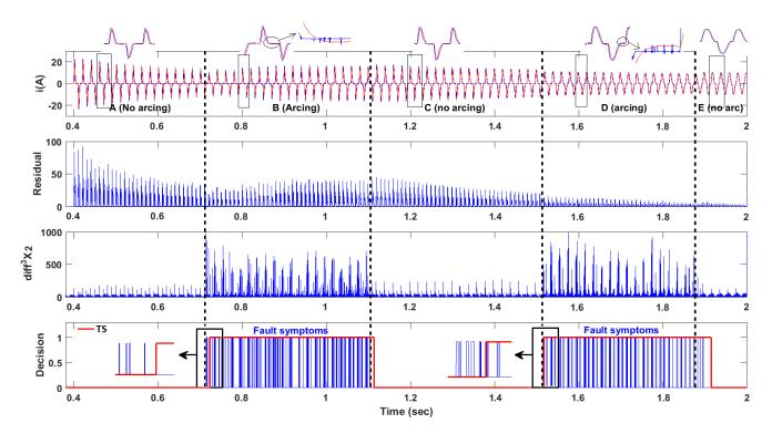
Figure 12: Sub-case 1: transient current of vacuum cleaner 2.
