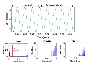
Figure 7: Residuals generation using different frequency rates.
