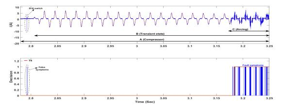
Figure 18: Transient current of a drill (with disruptive compressor).
