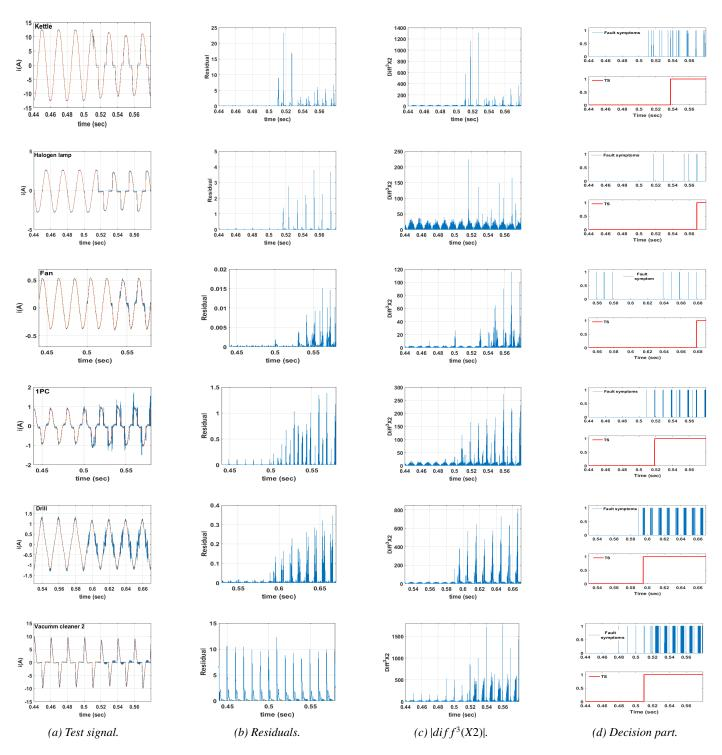
Figure 11: Fault detection in stationary operating mode.
