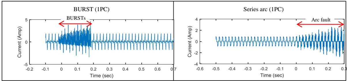
Figure 8. Currents comparison (BURSTS / series arc).
