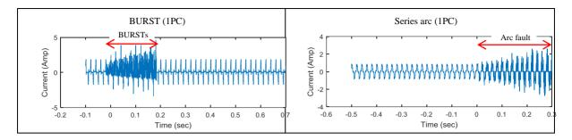
Figure 8. Currents comparison (BURSTs / series arc).
