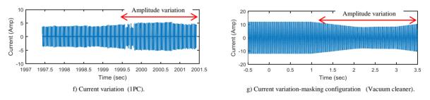
Figure 7. Current of the line considering differents EMI perturbations.
