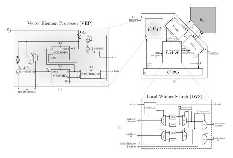
Fig. 2. (a) Architectures of the SOM-NoC's PE, (b) VEP and (c) LWS circuit
