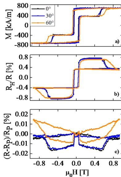
FIG. 4. Dependence of the magnetoresistance of a  $\text{Co}_{88}\text{Tb}_{12}(20 \text{ nm})/\text{Cu}(3.5)/\text{Co}_{74}\text{Tb}_{26}(20 \text{ nm})$  spin valve on the angle between the applied field and the perpendicular easy axis. (a) VSM hysteresis loops and (b) Hall resistance. (c) Four-point-probe CIP resistance (the field is always perpendicular to the current).
