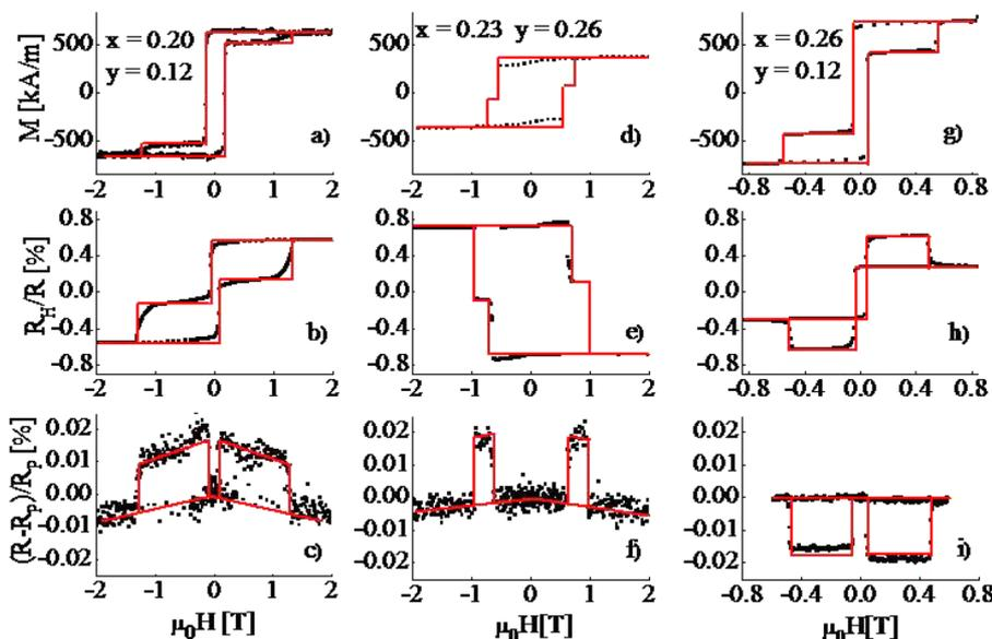
FIG. 3. SQUID hysteresis loops (a,d,g), Hall resistance (b,e,h) and four-point-probe CIP resistance (c,f,i) for a series of  $\text{Co}_{1-y}\text{Tb}_y(20 \text{ nm})/\text{Cu}(3.5 \text{ nm})/\text{Co}_{1-x}\text{Tb}_x$  spin valves: (a)–(c)  $x = 0.20$  and  $y = 0.12$ ; (d)–(f)  $x = 0.23$  and  $y = 0.26$ ; (g)–(i)  $x = 0.26$  and  $y = 0.12$ . Lines are guides to the eye.
