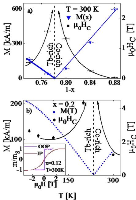
FIG. 1. Magnetization  $M$  and coercivity  $\mu_0 H_C$  of  $\text{Co}_{1-x}\text{Tb}_x$  (20 nm) alloys obtained from SQUID magnetometry: (a)  $M$  and  $\mu_0 H_C$  as a function of the Co concentration  $1-x$  at room temperature. (b)  $M$  and  $\mu_0 H_C$  as a function of temperature for a  $\text{Co}_{80}\text{Tb}_{20}$  alloy. Inset: In-plane (IP) and out-of-plane (OOP) hysteresis loop for a  $\text{Co}_{88}\text{Tb}_{12}$  alloy at room temperature. Lines are guides to the eye.
