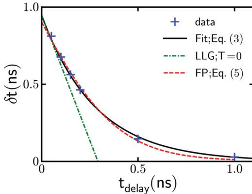
FIG. 2. (Color online)  $\delta t$  versus delay  $t_{\text{delay}}$ . The blue crosses are determined from the experimental data in Fig. 1. The black solid curve is an exponential fit to Eq. (3). The green dashed-dotted line is a calculation from the LLG equation for  $T = 0$ . The red dashed curve is a calculation based on a Fokker-Planck analysis [Eq. (8)].
