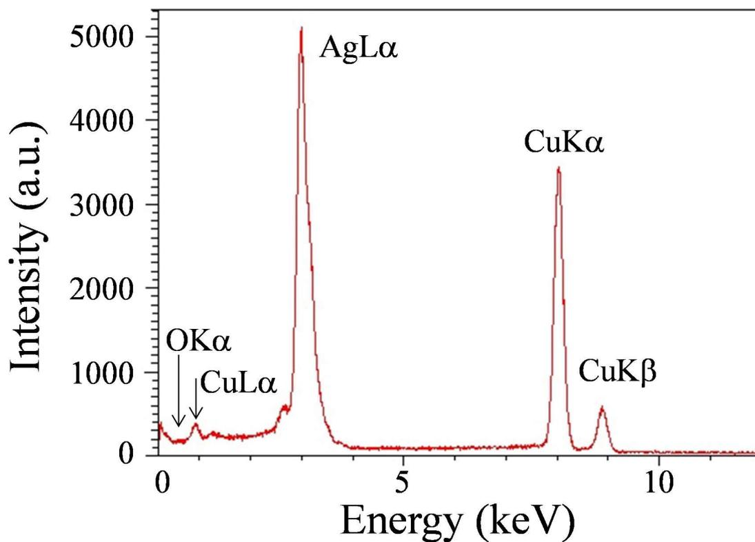
**Figure S1:** EDX spectrum corresponding to the object displayed in Fig. 2b. The oxygen peak is practically negligible. Quantitative analysis indicates it is 100 at.% pure silver. Copper is due to the TEM grid.
