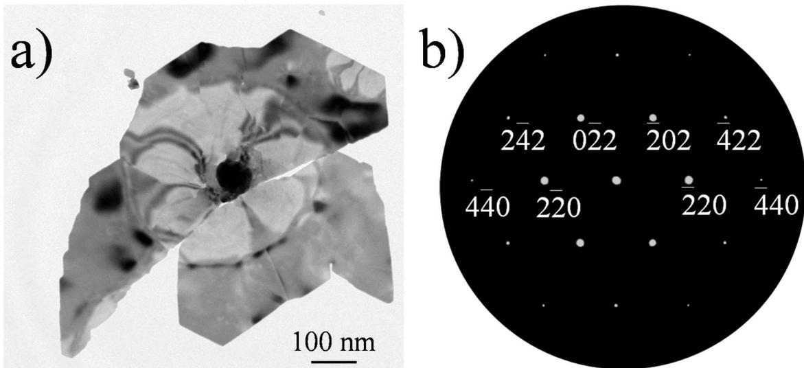
**Figure 6:** a) TEM images of two-dimensional nano-object produced from  $\text{Cu}_{28}\text{Ag}_{72}$  electrodes. b) Typical diffraction pattern of two-dimensional nano-object interpreted as the cubic  $\text{Ag}_{98.5}\text{Cu}_{1.5}$  phase (ref. 9016252 of the Crystallography Open Database).
