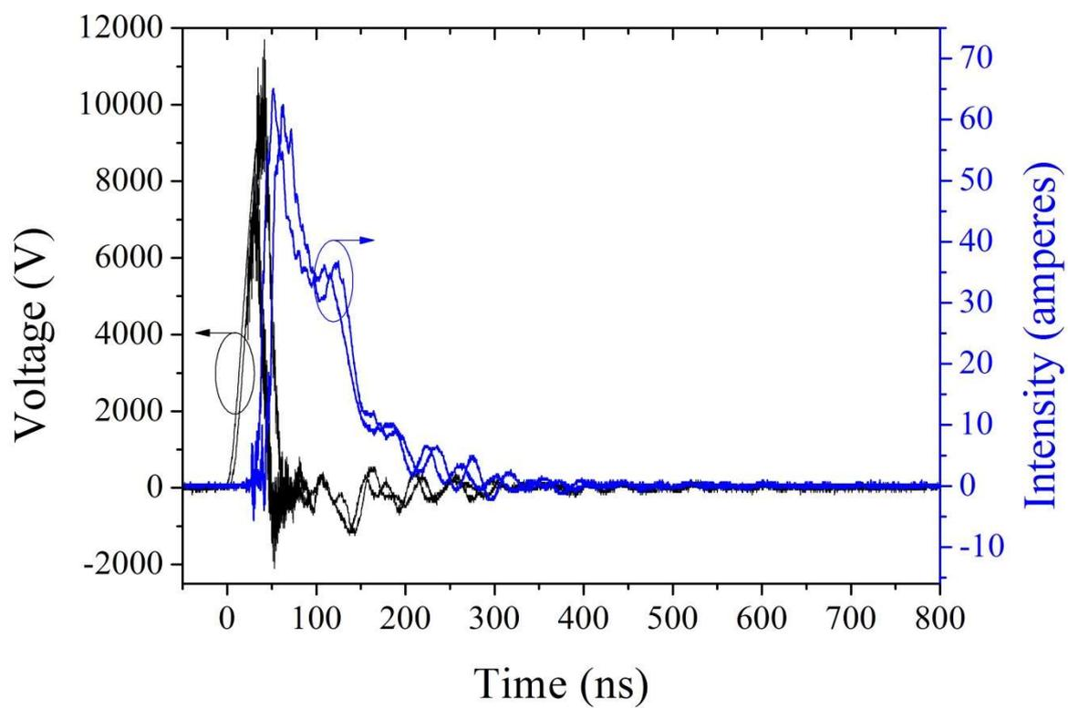
**Figure S6:** Time-evolution of voltage and current signals for Ag and CuAg electrode pairs. Signals are almost identical. The energy deposited varies by less than 1.6% from one situation to the other.
