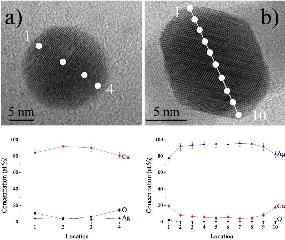
**Figure 5:** High-resolution TEM images showing a) a spherical copper-rich nanoparticle with its composition profile determined over 4 points, b) a faceted silver-rich nanoparticle with its composition profile determined over 10 points. The average composition of each particle made over all points but the two outermost is  $(\text{Cu}_{90.9}\text{Ag}_{4.1}\text{O}_{5.0})$  and  $(\text{Ag}_{93.8}\text{Cu}_{6.2})$ .
