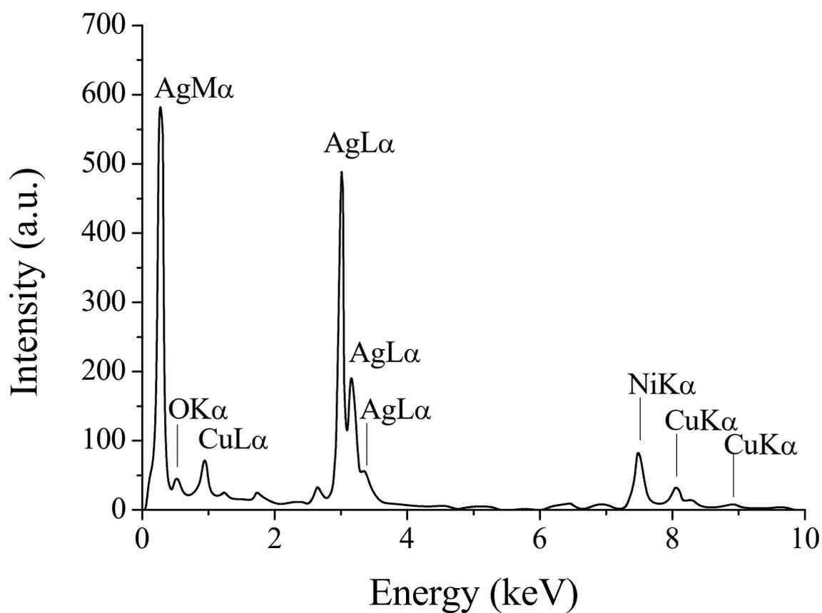
**Figure S3:** EDX spectrum corresponding to the object displayed in Fig. 7a. Quantitative analysis indicates that it is  $\text{Ag}_{85.5}\text{Cu}_{5.5}\text{O}_{9.0}$ . The  $\text{K}\alpha$  line of nickel is due to the grid.
