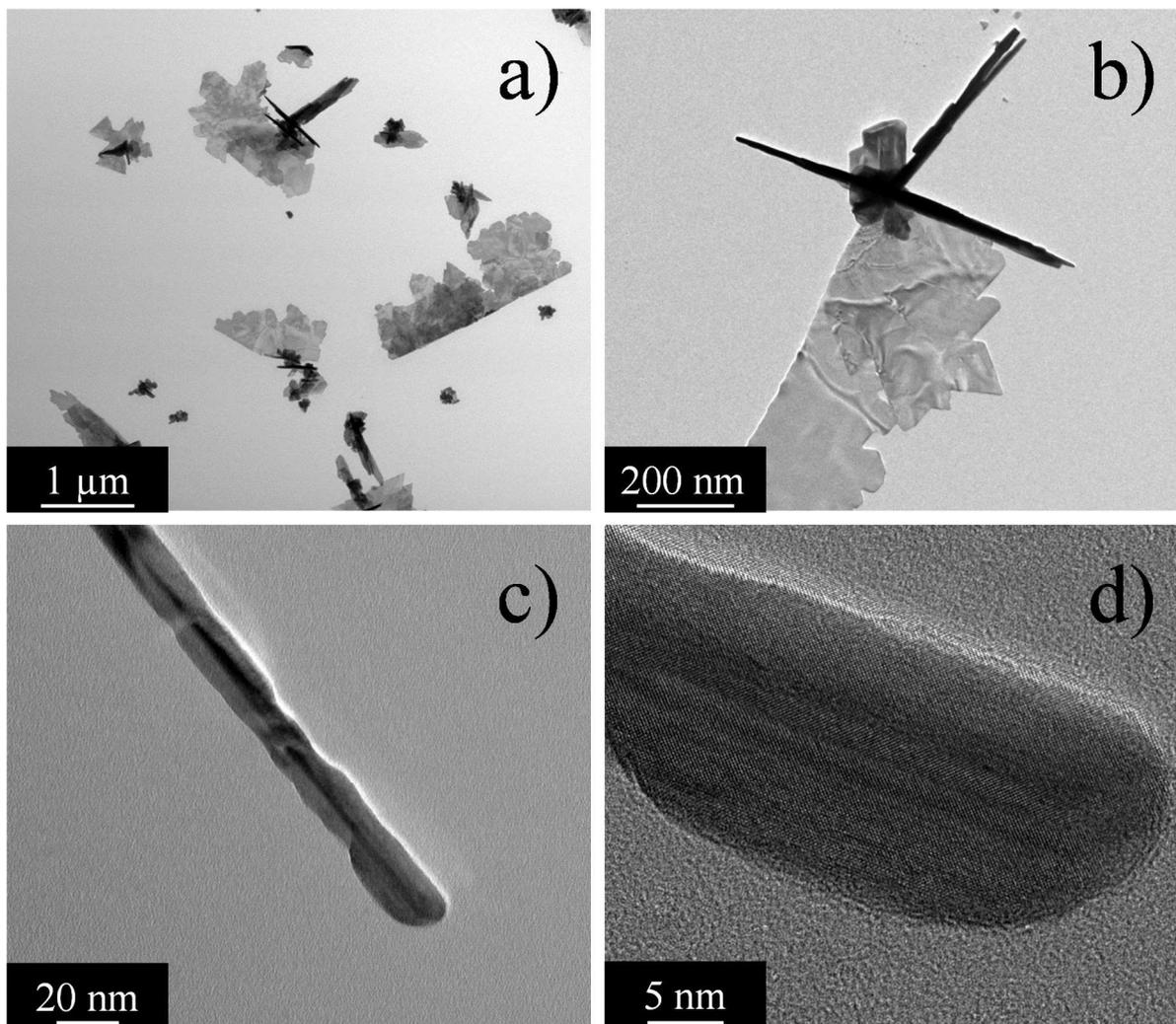
**Figure 9:** a) Large view TEM image showing the presence of nanorods associated with sheets. b) Close view TEM image showing nanorods attached together. c) Overall view of a single wire. d) High-Resolution TEM image of a nanorod showing its crystalline structure.
