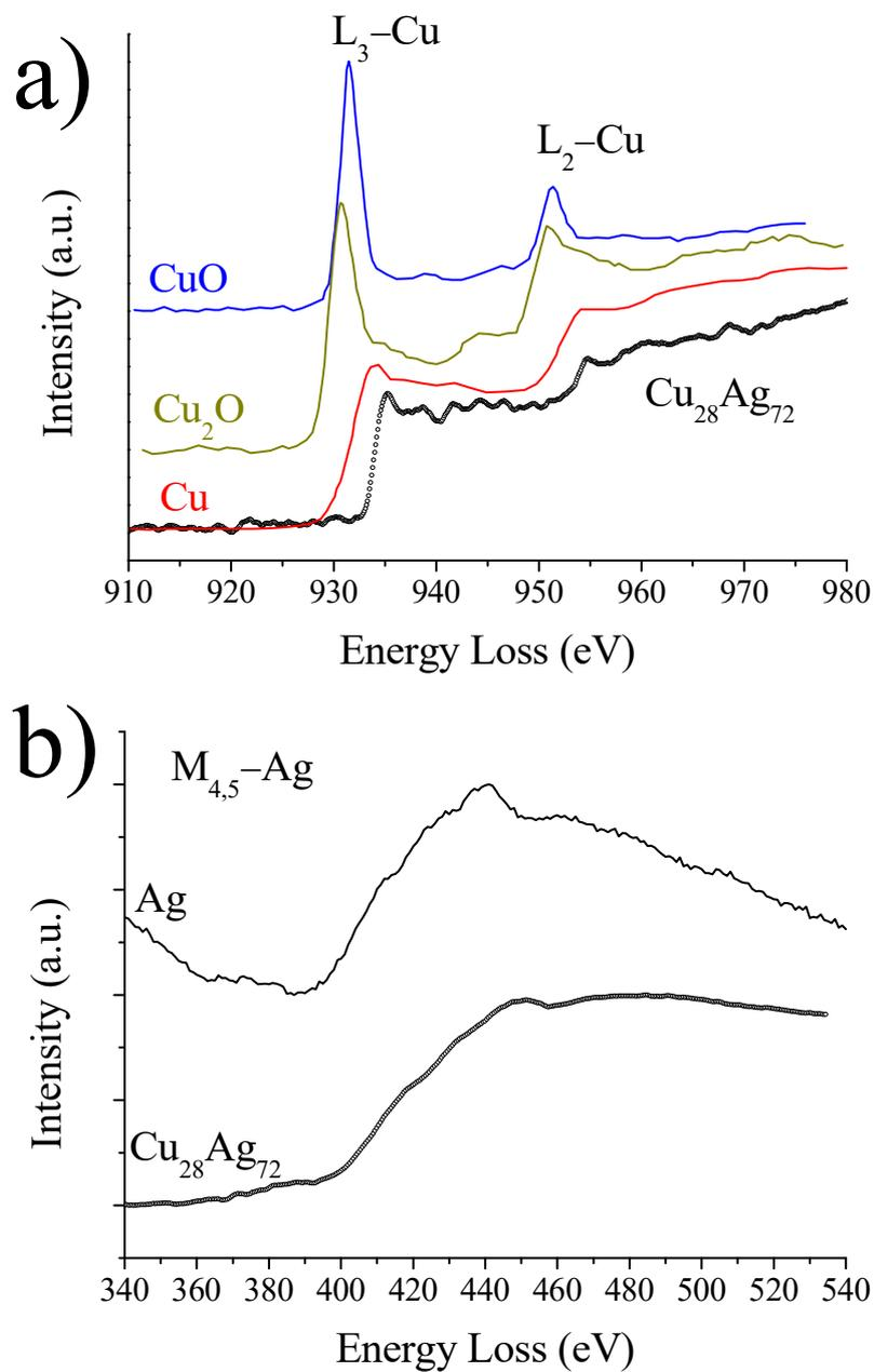
**Figure S2:** Electron Energy Loss Spectroscopy near-edge fine structures for the Cu L<sub>2,3</sub>. b) Electron Energy Loss Spectroscopy near-edge fine structures for the Ag M<sub>4,5</sub>. Cu, CuO, Cu<sub>2</sub>O and Ag spectra are given as reference.
