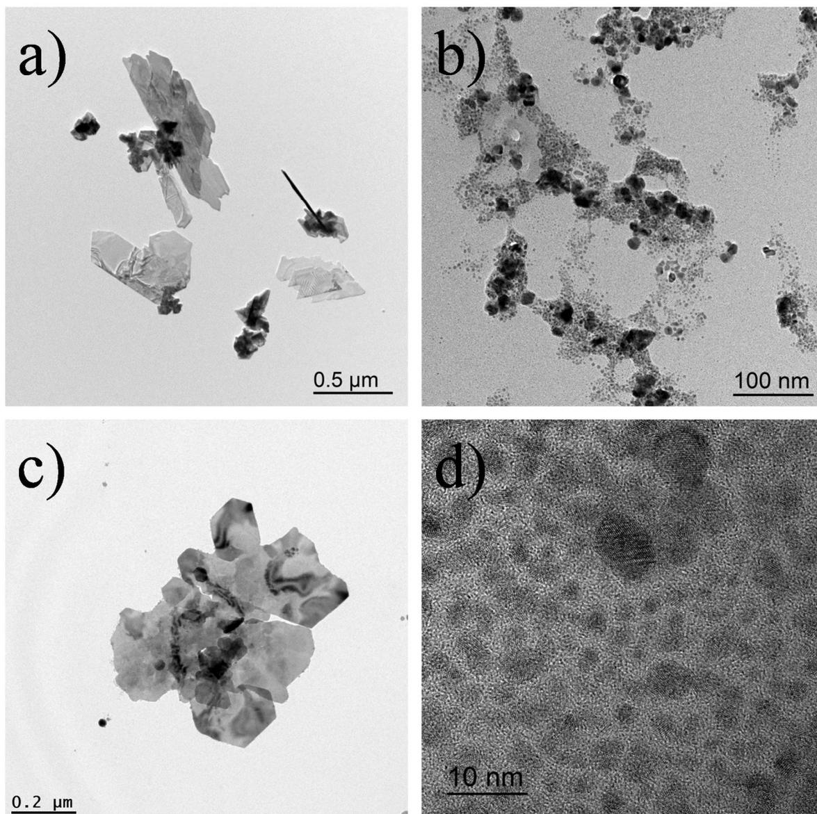
**Figure 4:** a) Low-resolution TEM image of a set of two-dimensional sheets synthesized between  $\text{Cu}_{28}\text{Ag}_{72}$  electrodes immersed in liquid nitrogen and observed after air exposure. The presence of nanorods is sometimes observed. b) Nanoparticles with two size distributions. c) Magnification of an isolated sheet. d) High-resolution image of small-size nanoparticles showing their crystalline structure.
