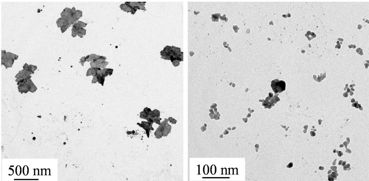
**Figure 1:** a) Copper oxide (CuO) nanoparticles synthesized between two Cu electrodes immersed in liquid nitrogen and observed after air exposure at two scales by TEM. b) Silver (Ag) sheets and nanoparticles synthesized between two Ag electrodes immersed in liquid nitrogen and observed after air exposure at two scales by TEM.
