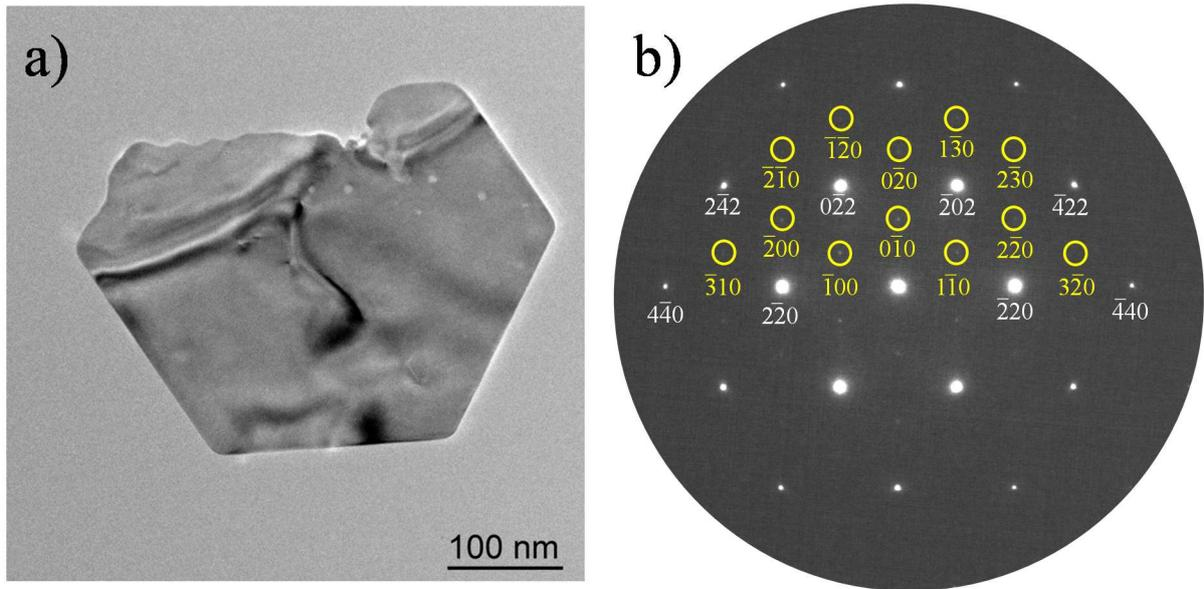
**Figure 11:** a) Studied silver-rich single nanosheet. b) Corresponding diffraction pattern showing the presence of two different phases. The circled spots have low intensity and are indexed as the Ag<sub>98.5</sub>Cu<sub>1.5</sub> hexagonal phase. The other ones are indexed as the cubic phase of the same alloy.
