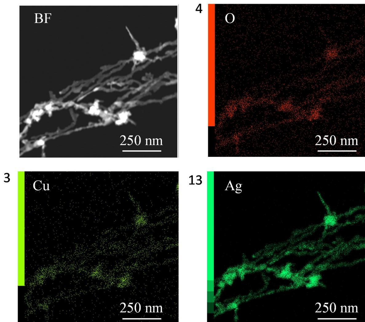
**Figure S4:** X-mapping of one-dimensional objects shown in the Bright Field image (same as **Fig.11** right). Ag, O and Cu maps are depicted together with their intensity colour scales whose maximum values are indicated by the given numbers.
