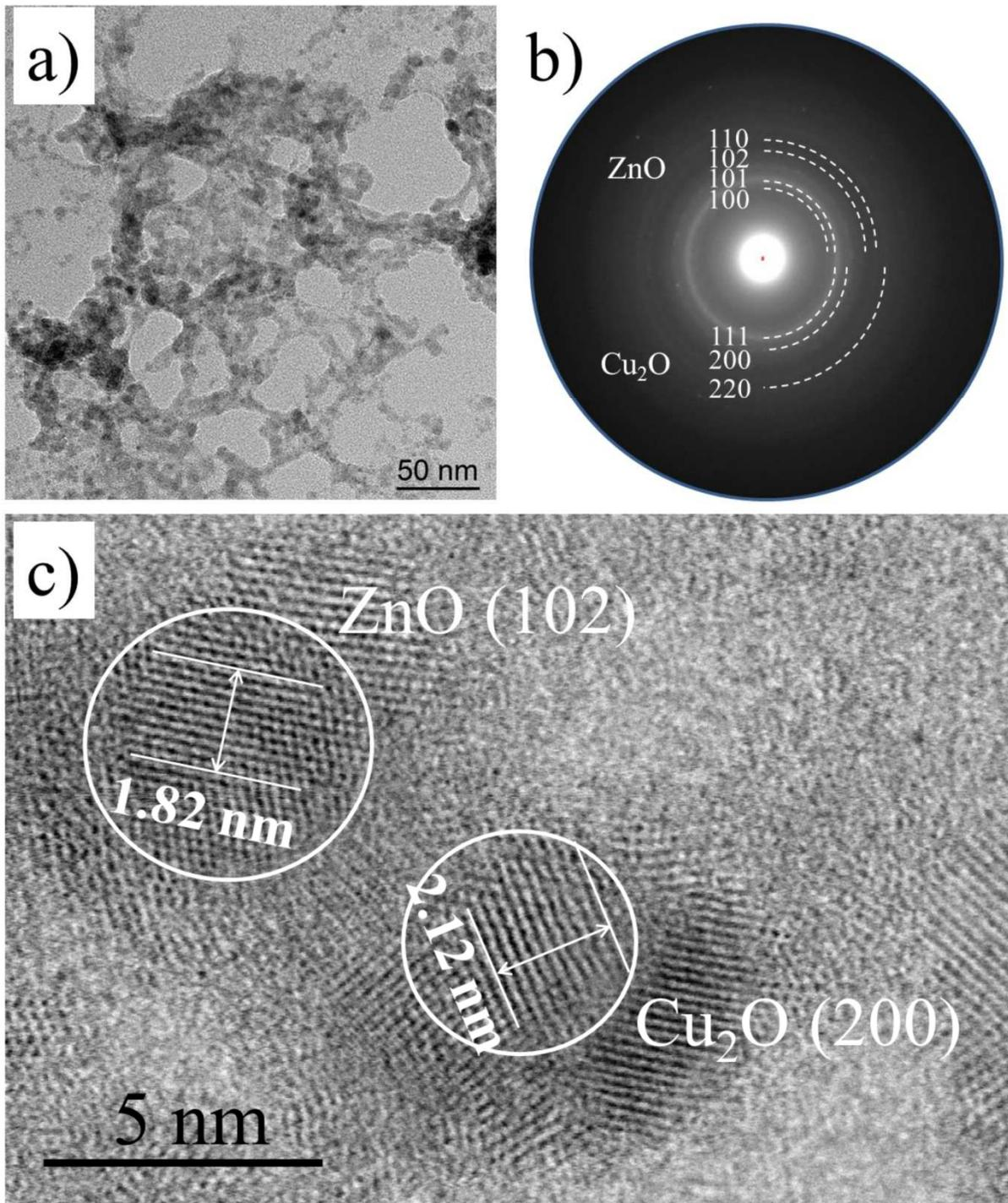
**Figure 2:** a) Low magnification bright field TEM images of NPs synthesized with brass electrodes. b) Corresponding Selected Area Electron Diffraction pattern showing the simultaneous presence of Cu<sub>2</sub>O and ZnO. c) High resolution TEM images showing crystalline ZnO and Cu<sub>2</sub>O NPs. The interplanar distance is measured from 10 consecutive planes, as depicted by arrows.
