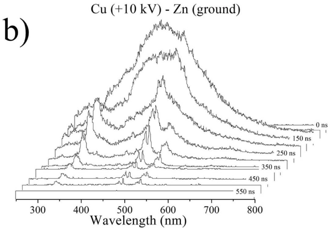
**Figure 9:** Time evolution of optical emission spectra recorded every 50 ns when both electrodes are made of brass a) and when high voltage is applied to the copper electrode, the zinc electrode being grounded.
