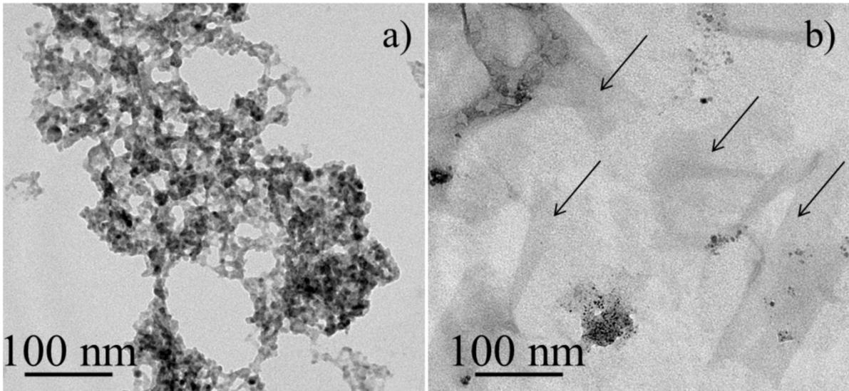
**Figure 1:** a) Copper oxide (CuO) nanoparticles synthesized between two Cu electrodes immersed in liquid nitrogen and observed after air exposure by TEM. b) Zinc oxide (ZnO) sheets (depicted by arrows) and nanoparticles synthesized between two Zn electrodes immersed in liquid nitrogen and observed after air exposure by TEM.
