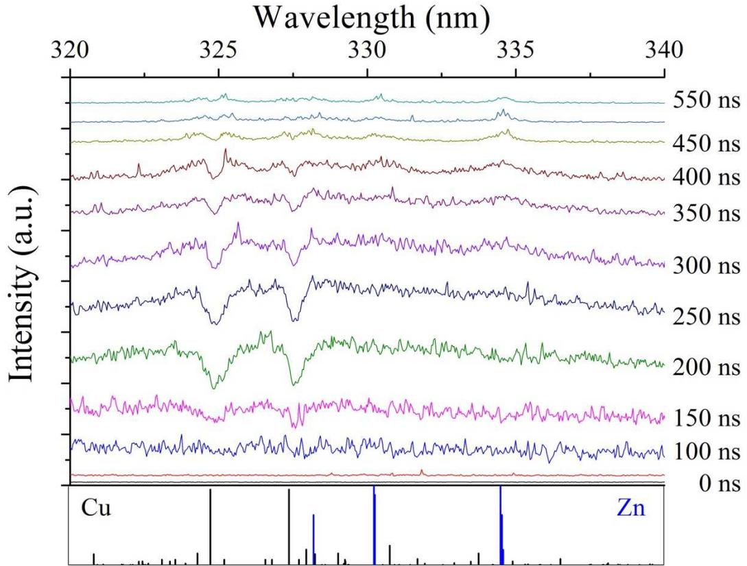
**Figure 10:** Self-absorption of Cu resonant lines observed in the case of brass electrodes with a  $1,200 \text{ g mm}^{-1}$  grating. Copper (resp. zinc) lines referenced in NIST [16] are shown by vertical black (resp. blue) threads whose length is proportional to the relative intensity of the line. Data at 0, 50 and 100 ns, where no self-absorption is noticed, are not reported to better depict the time evolution of self-absorbed lines.
