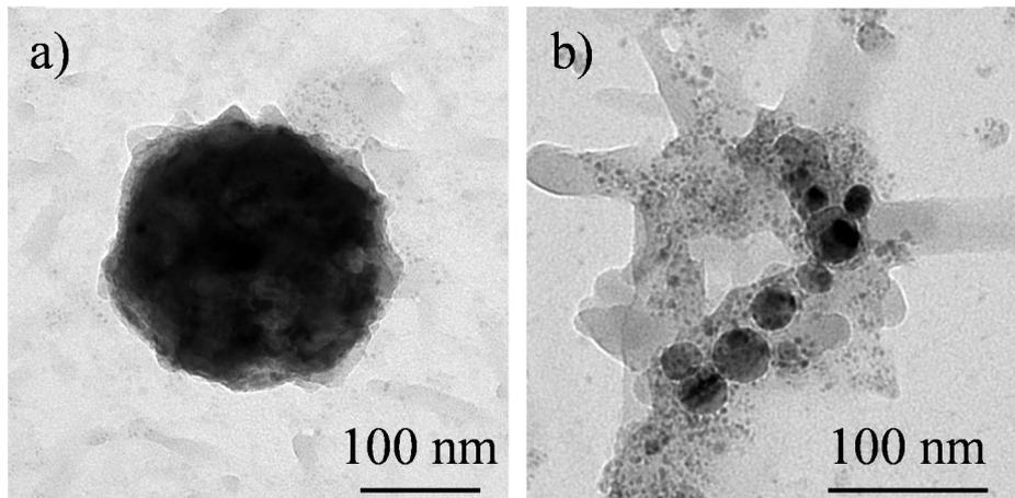
**Figure 12:** Nanoparticles synthesized from  $\text{Cu}_{63}\text{Zn}_{37}$  electrodes in a) water and b) ethanol.
