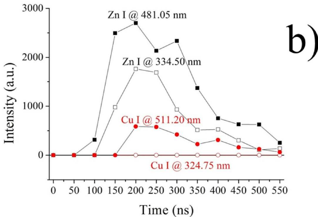
**Figure 11:** Time evolution of selected lines a) when both electrodes are made of brass a) and when high voltage is applied to the copper electrode, the other zinc electrode being grounded.
