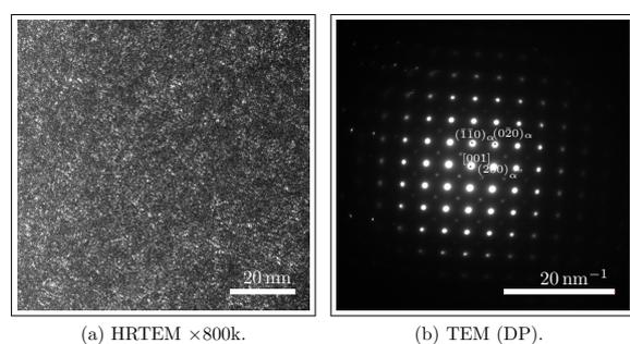
Figure 10: Same sample as Fig. 9 but after tempering at 573 K: (a) high resolution (HRTEM) detail of the  $\text{Fe}_{16}\text{N}_2$  nano-precipitates, (b) SAED oriented according to along  $[001]_{\alpha}$ .
