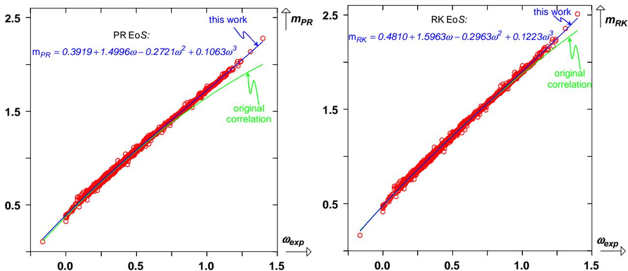
**Figure 1.** Correlation of optimized  $m$  parameter against  $\omega_{exp}$  for both the PR and RK EoS. Comparison between the original correlation and the one determined in this work. Each of the 1721 open circles represent a pure compound.
