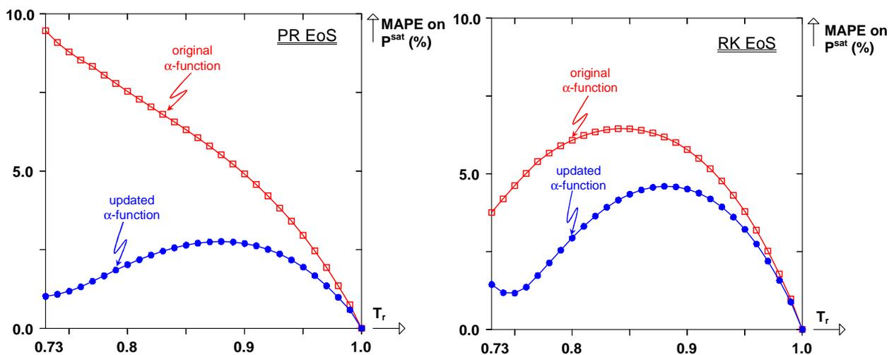
**Figure 3.** MAPE on  $P^{sat}$  for heavy molecules (see **Table 3**) plotted against the reduced temperature for PR (left) and RK (right) EoS. (□) Original  $\alpha$ -function, (●) Updated  $\alpha$ -function.
