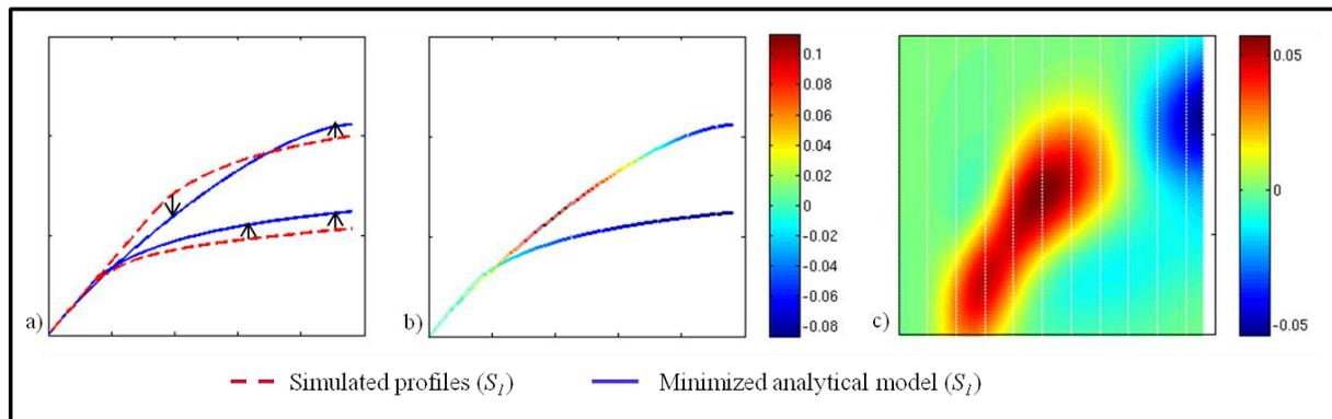
**Fig. 9 – (a) Error computed between simulation profiles and analytical profile for two models belonging to  $\mathcal{S}_1$ . (b) Mapping error on analytical model. (c) Interpolation of the error on the entire plot domain to create an error map.**
