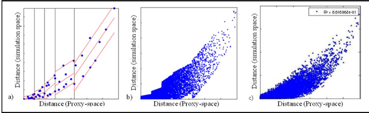
**Fig. 4– (a) Cross plot of full flow simulation distances vs. proxy distances for  $\mathcal{S}_1$ . Vertical lines represent domain borders. Red lines represent domain regression surrounded by the quantiles Q10 and Q90 of the residuals. (b) Cross plot of the reconstructed full flow simulation distances for  $\mathcal{S}_2$  (obtained by random draw as explained in the text) vs. proxy distances. (c) True cross plot of full flow simulation distance vs. proxy distance, used as benchmark**
