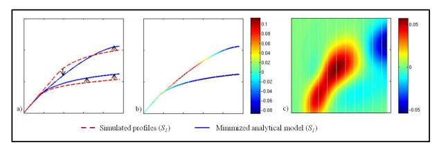
Fig. 9 – (a) Error computed between simulation profiles and analytical profile for two models belonging to  $S_1$ . (b) Mapping error on analytical model. (c) Interpolation of the error on the entire plot domain to create an error map.
