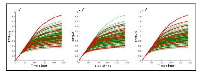
Fig. 3 – Examples of models selection. The red curves represent the 10 selected models while the green curves represent the other models. The vertical axis represents the cumulative oil production or Field Oil Production Total (FOPT)
