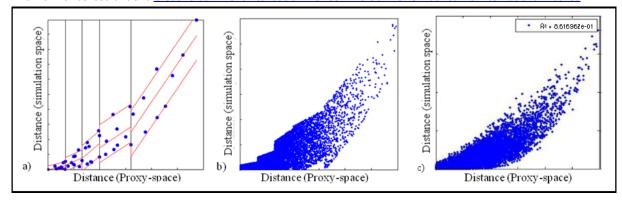
Fig. 4– (a) Cross plot of full flow simulation distances vs. proxy distances for  $\mathcal{S}_1$ . Vertical lines represent domain borders. Red lines represent domain regression surrounded by the quantiles Q10 and Q90 of the residuals. (b) Cross plot of the reconstructed full flow simulation distances for  $\mathcal{S}_2$  (obtained by random draw as explained in the text) vs. proxy distances. (c) True cross plot of full flow simulation distance vs. proxy distance, used as benchmark
