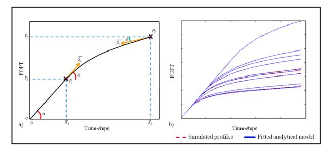
Fig. 5 – a) Graphical view of the analytical model and parameters of analytical oil recovery profiles. b) Result of least-squares fit of the analytical model (red curves) to production profiles obtained by flow simulation (blue curves).
