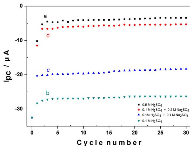
**Figure 5.** Variation of the intensity of the first cathodic peak currents obtained after transferring an electrode pretreated for 50 successive CV scans in 0.5 mM  $[\text{SiW}_{12}\text{O}_{40}]^{4-}$  to a POM-free solution,
