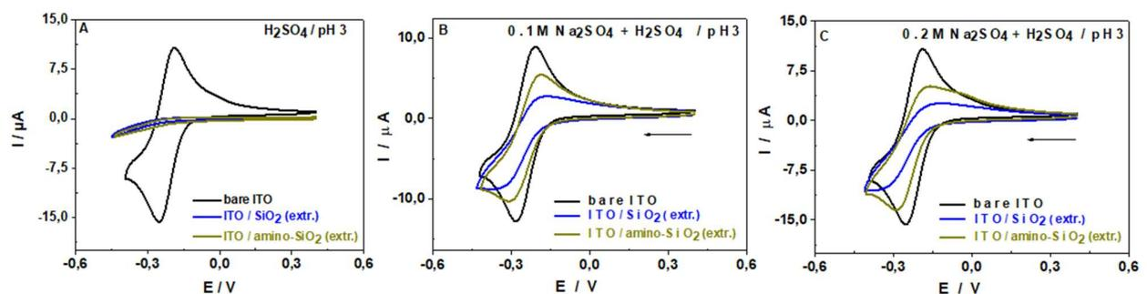
**Figure 7.** Cyclic voltammograms recorded in a solution containing  $5.0 \times 10^{-4}$  M  $[\text{SiW}_{12}\text{O}_{40}]^{4-}$  and 0.001 M  $\text{H}_2\text{SO}_4$  alone (A), or with 0.1 M  $\text{Na}_2\text{SO}_4$  (B) or 0.2 M  $\text{Na}_2\text{SO}_4$  (C), using bare ITO electrode (black), ITO covered with a mesoporous silica film after surfactant extraction (blue), and an amino-functionalized silica film on ITO (dark green).
