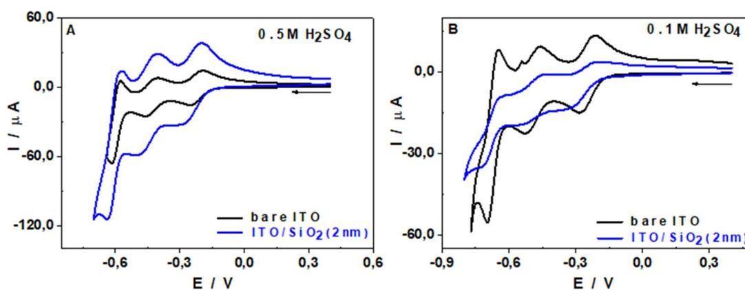
**Figure 3.** Cyclic voltammograms recorded in a solution containing  $5.0 \times 10^{-4}$  M  $[\text{SiW}_{12}\text{O}_{40}]^{4-}$  and H<sub>2</sub>SO<sub>4</sub> at concentrations adjusted to fix pH values at 0.3 (A) or 1.0 (B) using bare ITO electrode (black) and ITO covered with a mesoporous silica film after surfactant extraction (blue); a control experiment performed prior to surfactant extraction is also shown in red on part A of the figure.
