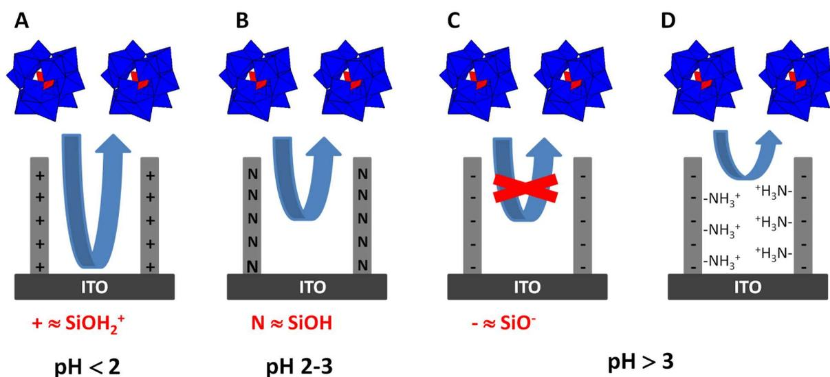
**Scheme 2.** Schematic illustration of the surface charge of silica nanochannels as a function of pH and their effect on the film permeability to the anionic redox probes. A) pH < pI: Positive charge density. B) pH = pI: Neutral silica. C) pH > pI: Negative charge density. D) Amino-functionalized silica film at pH > pI (protonated at pH lower than the pKa of ~10).
