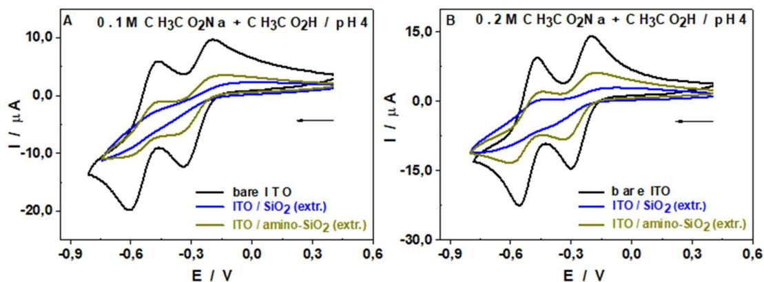
**Figure 7.** Cyclic voltammograms of  $5.0 \times 10^{-4}$  M  $[\text{SiW}_{12}\text{O}_{40}]^{4-}$  in acetate buffer at pH 4.0 (0.1 M (A) or 0.2 M (B)), using bare ITO electrode (black) and ITO covered with a mesoporous silica film after surfactant extraction (blue).
