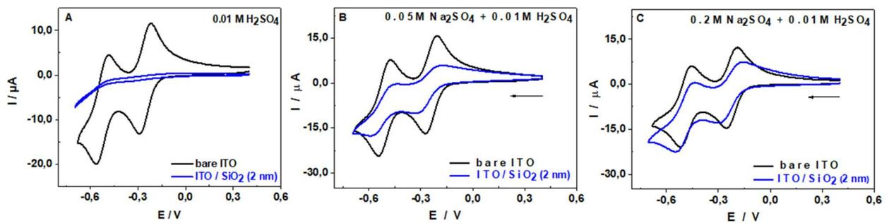
**Figure 6.** Cyclic voltammograms recorded in a solution containing  $5.0 \times 10^{-4}$  M  $[\text{SiW}_{12}\text{O}_{40}]^{4-}$  at pH 2 (0.01 M  $\text{H}_2\text{SO}_4$ , A) to which increasing amounts of  $\text{Na}_2\text{SO}_4$  have been added (0.05 M (B) and 0.2 M (C)), using bare ITO electrode (black) and ITO covered with a mesoporous silica film after surfactant extraction (blue).
