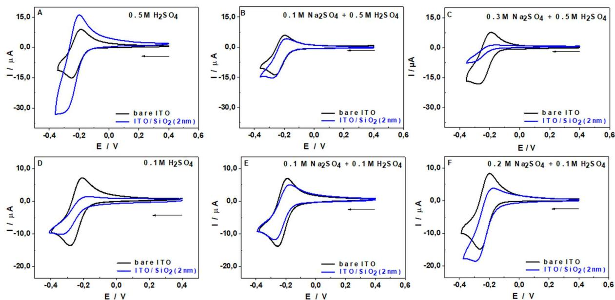
**Figure 4.** Cyclic voltammograms recorded in a solution containing  $5.0 \times 10^{-4} \text{ M } [\text{SiW}_{12}\text{O}_{40}]^{4-}$  and  $\text{H}_2\text{SO}_4$  at concentrations adjusted to fix pH values at 0.3 (A-C) or 1.0 (D-F) and  $\text{Na}_2\text{SO}_4$  at selected concentrations (see on plots) to get various ionic strengths, using bare ITO electrode (black) and ITO covered with a mesoporous silica film after surfactant extraction (blue). Electrolyte media
