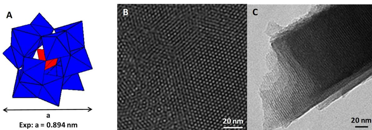
**Figure 1.** A) Representative structure of the heteropolyanion studied:  $[\text{SiW}_{12}\text{O}_{40}]^{4-}$ . B, C) Transmission electron micrographs of the vertically-oriented silica thin films: top-view (B) and cross-section (C).
