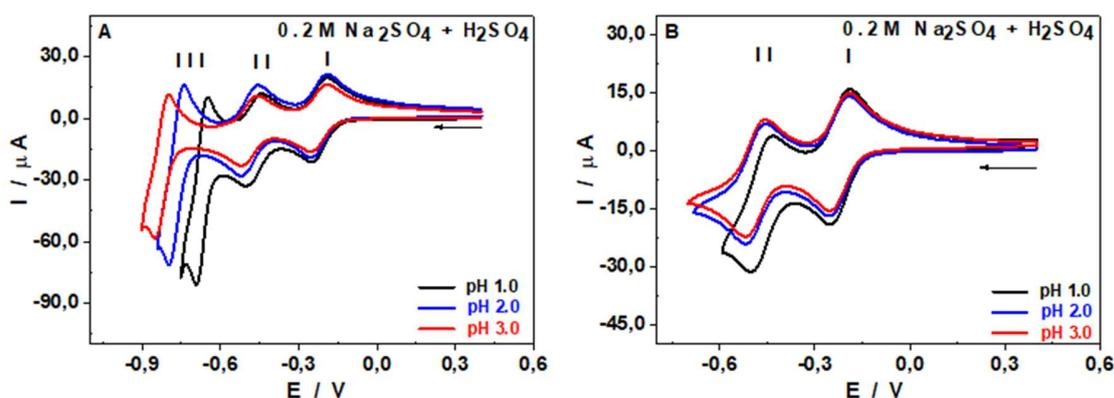
**Figure 2.** Cyclic voltammograms recorded on bare ITO electrode in a solution containing  $5.0 \times 10^{-4}$  M [SiW<sub>12</sub>O<sub>40</sub>]<sup>4-</sup> and 0.2 M Na<sub>2</sub>SO<sub>4</sub> + H<sub>2</sub>SO<sub>4</sub> at different concentrations adjusted to fix pH values at 0.3 (black line), 1.0 (red line), 2.0 (blue line) and 3.0 (green line). Part A represents the whole potential window while part B is restricted to that of the two first redox processes.
