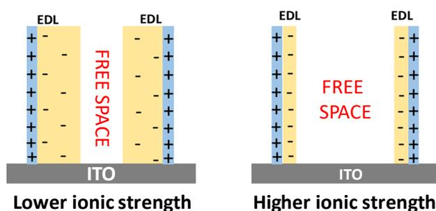
**Scheme 1.** Schematic representation of the nanochannels in highly acidic medium (where the low pH induces positive charges on the silica walls) as a function of the ionic strength.
