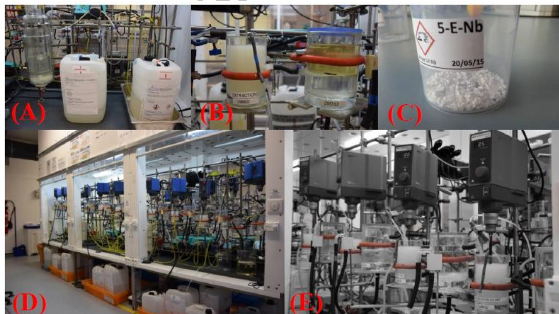
Figure S 1 : Pictures of the Nb-Ta separation pilot campaign. (A) Alkaline feed solution containing Nb and Ta. (B) Mixer-settlers corresponding to the Nb-Ta co-extraction step. (C) Purified Nb oxide. (D) and (E) Views of the process.
